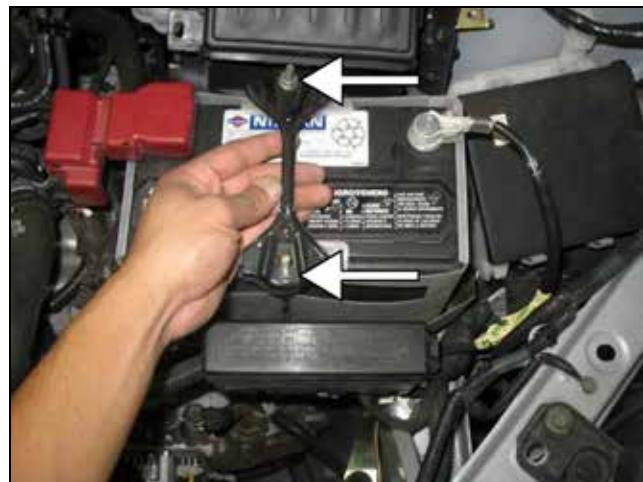
f. Loosen both nuts securing the J-hooks. Remove the J-hooks and battery bracket.
