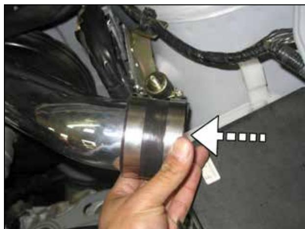
i. Attach the coupler and #40 hose clamps to the installed inlet pipe.
