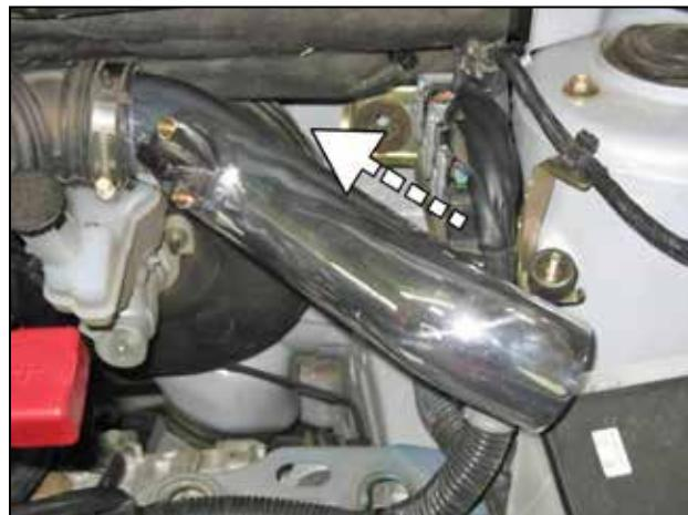
g. Insert the inlet pipe as shown.
