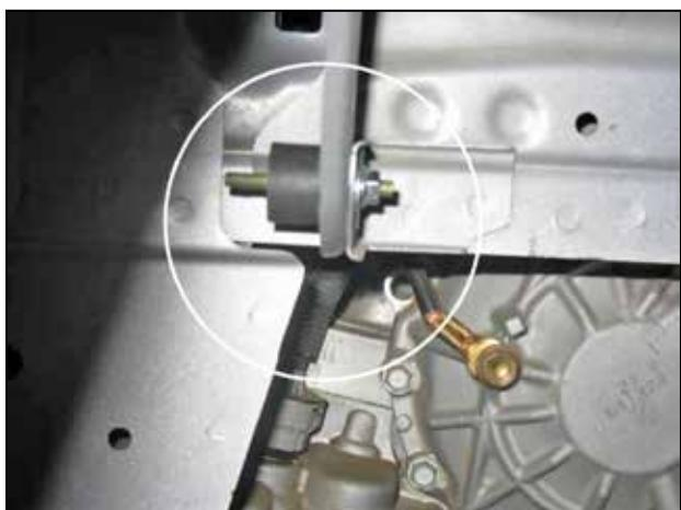
h. Attach the 1" rubber mount in the fender well.
