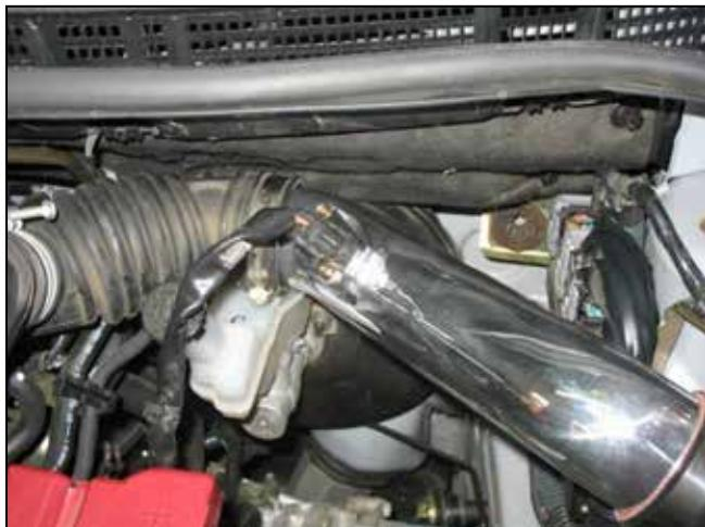
n. Plug in the MAF sensor connector.
