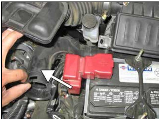
e. Unclip and remove the lower air ducting from the air box.
