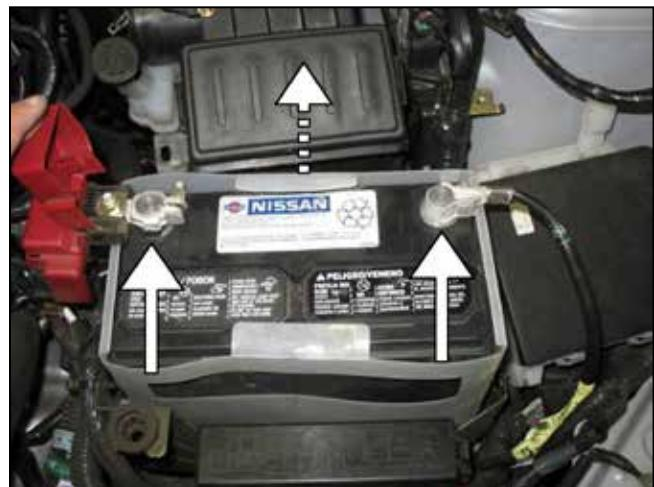
h. Loosen and remove both battery terminals. Remove the battery. With the battery removed, pull the air box out from the mounting grommets.
