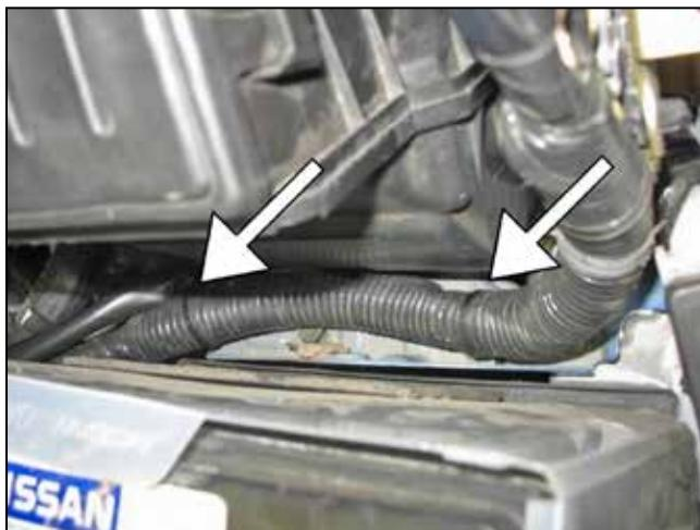
g. Cut the wire tie securing the ECU wire harness to the battery bracket.
