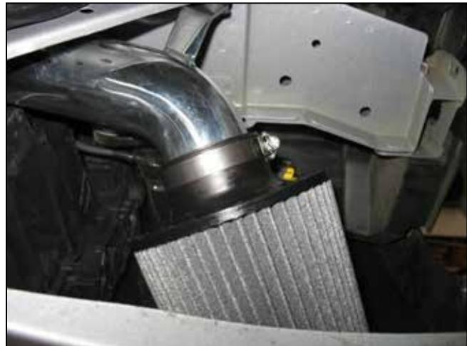
m. Attach the air filter element and secure with #44 hose clamp.
