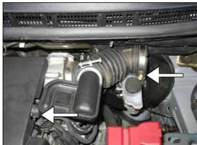
b. Insert the tree mount zip ties into the factory location on the batter bracket. Secure the ECU wire harness to the bracket. Cut off excess tie.
