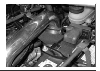
g. Install the 90-degree rubber elbow onto the throttle body with the supplied hose clamps. Install the upper intake pipe, securing the upper section of the intake pipe into the rubber elbow and the lower section of the pipe to the air bypass valve.
