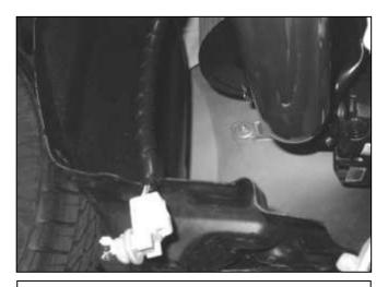
d. Disconnect the side marker lamp. Wrap the wires with the supplied helical wrap, then reconnect the side maker lamp.
