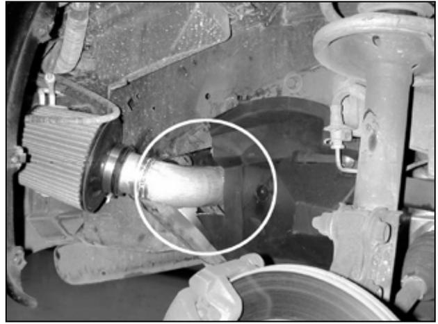
f. Attach the inner fender liner to determine where it will make contact with the intake pipe. The inner fender liner will need to be trimmed to clear the intake pipe. Once the liner is trimmed and provides adequate clearance, install the liner and the hardware needed to secure it in place.
