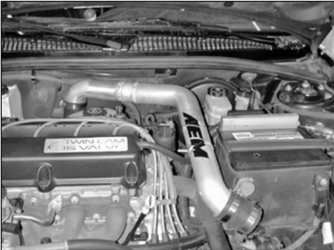
b. Attach the upper intake pipe with the provided couplers and hose clamps.
