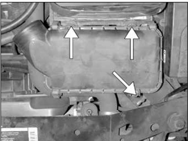
c. Remove the 3 - 10mm bolts securing the air box in place.
