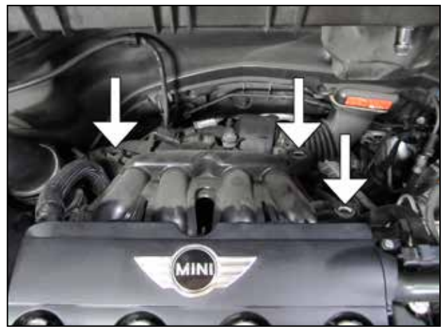
d. Pull up on the stock air box assembly carefully until it pops free from the 3 rubber mounting grommets on the intake manifold. Make sure all 3 rubber grommets stay in the intake manifold.
