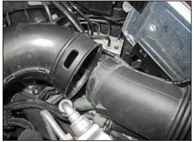
f. To completely remove the air box assembly, disconnect the air box inlet elbow (left) from the stock intake tube (right) by squeezing on the intake tube and pulling it free from the 4 locking slots in the intake elbow.
