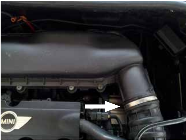
a. Loosen the hose clamp connecting the intake tube to the stock air box.
