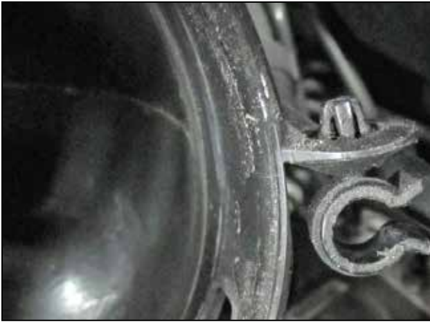
e. Unclip the plastic vacuum line from the lower intake elbow.
