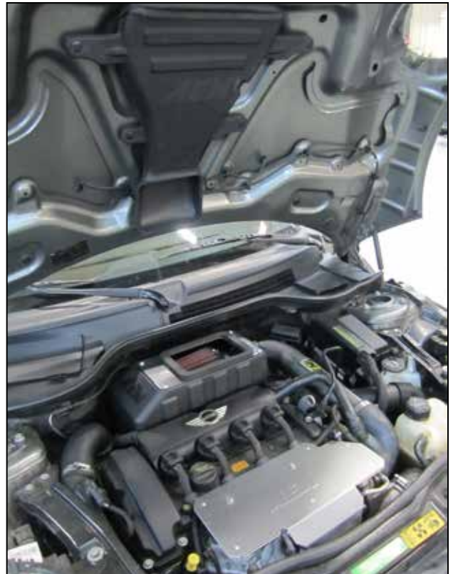
AEM® Cold Air Intake installed
