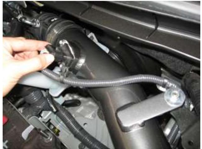
h. Install the MAF sensor connector onto the MAF sensor that was removed in 1a and reinstall fender well liner and wheel in reversed order outlined in step 2h.
