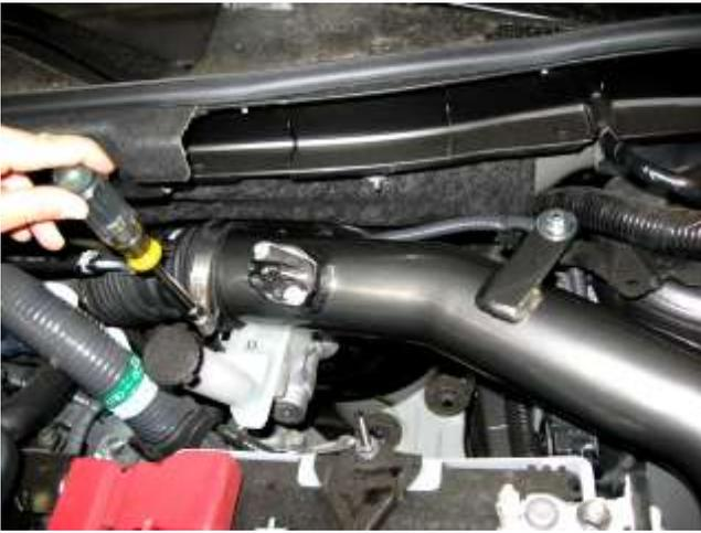
e. Position the AEM tube inside the stock intake hose and align the bracket with the rubber bushing. Tighten the hose clamp and the provided M6 nut/washer.
