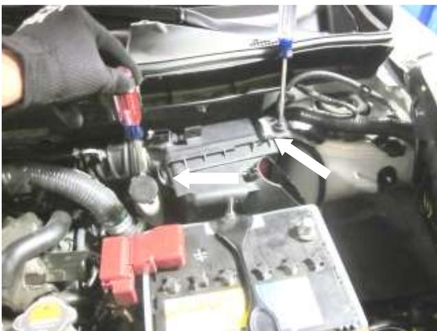
c. Loosen the hose clamp, remove the M6 bolt, and disconnect the two latches securing the air box lid to the base.
