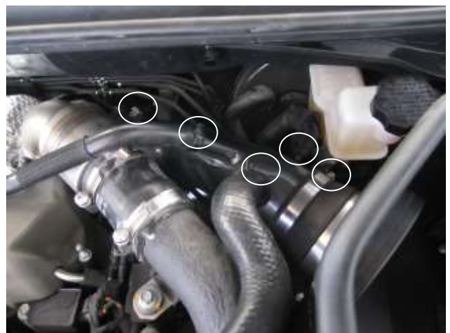
j. Install the AEM intake tube (2-1513C) into the two couplers. Tighten both hose clamps. Install all three of the hoses onto the tube and re-install the spring clamps to secure them that were removed in 2c.
