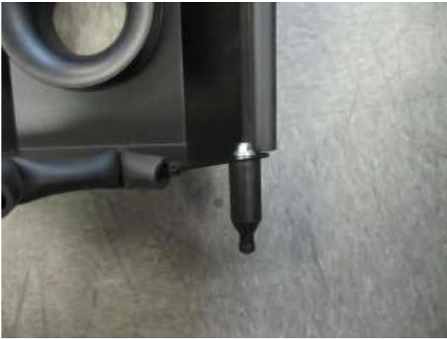
e. Install the standoff (06532) with the bolt (08318) and washer (08272) onto the heat shield as shown.
