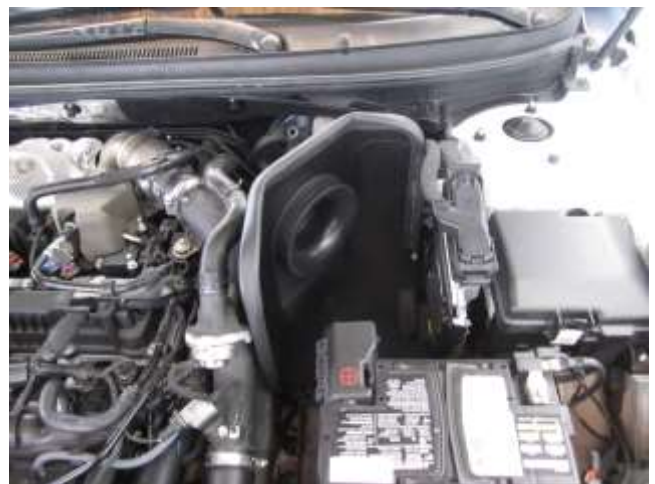
h. Install the completed heat shield into the vehicle aligning the 2 slots in the front to the previously installed mounts. Push down to secure the stand off.
