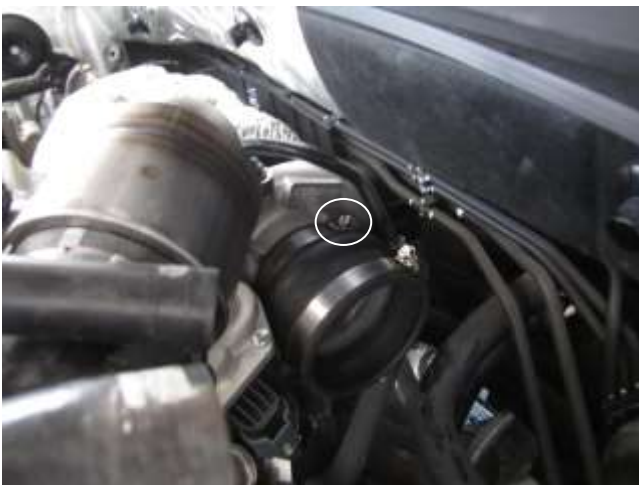
g. Install the hump hose (5-574) onto the turbo with the supplied hose clamps (9440 & 9448). Tighten the hose clamp closest to the turbo at this time.
