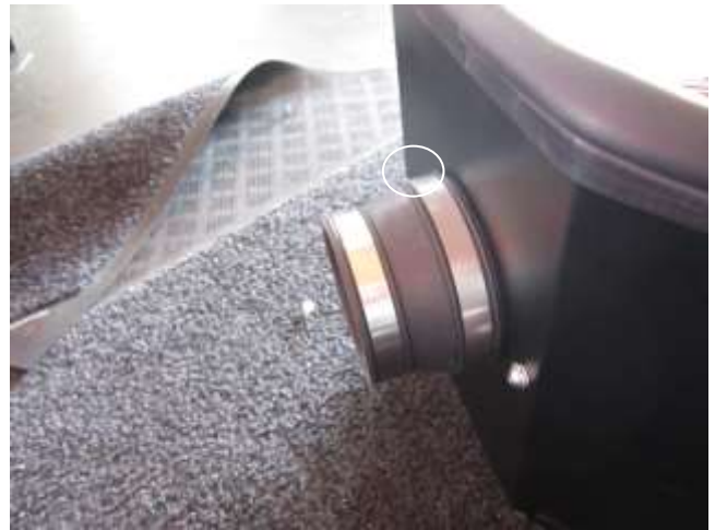
f. Install the hose adapter (5-1046) onto the filter adapter with hose clamps (9448 & 9456). Tighten the hose clamp closest to the heat shield at this time.
