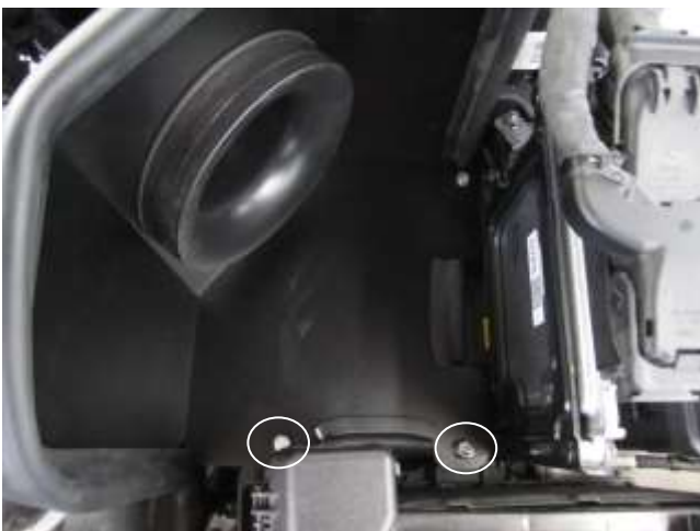
i. Install a washer (08275) and nut (07529) onto the rubber mount, shown on the right. Then install the bolt (08373), 2 washers(08275), and nut (07529) to secure the heat shield to the bracket. Ref. Exploded View
