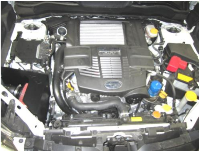
k. AEM intake system installed.
