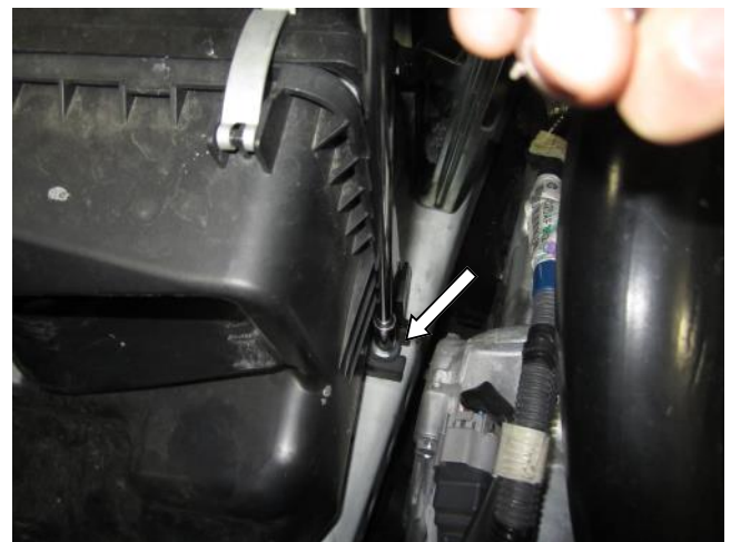
d. Remove the bolt that secures the air box to the engine bay and set aside for later use with AEM heat shield.
