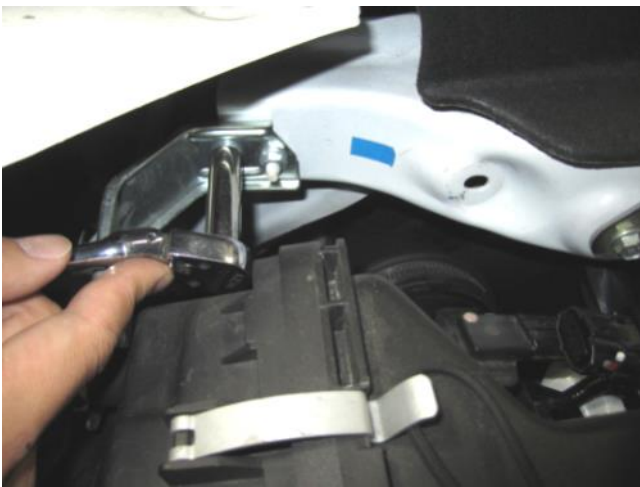
c. Remove the two nuts on the fender that secure the bracket for the air box.
