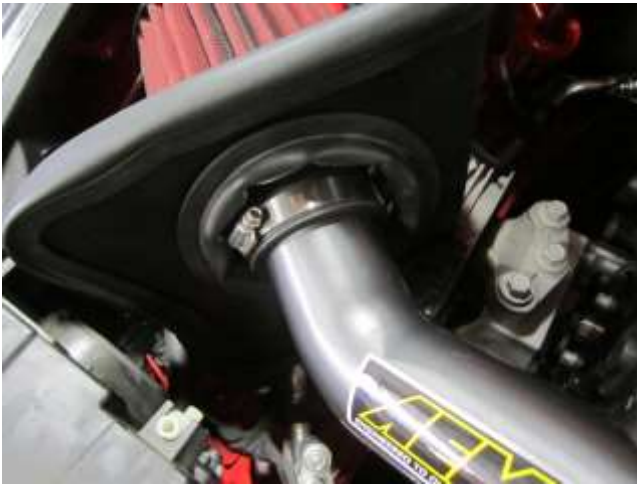
i. Install the AEM intake tube into the filter. Note: Do not fully tighten clamp at this time.
