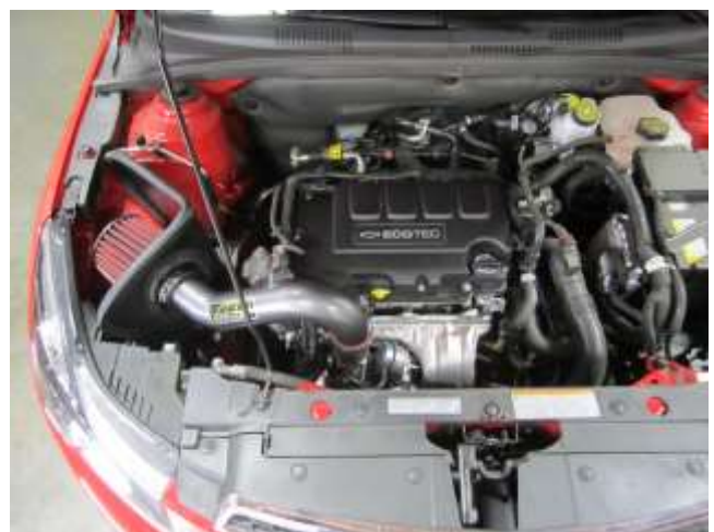
AEM INTAKE INSTALLED
