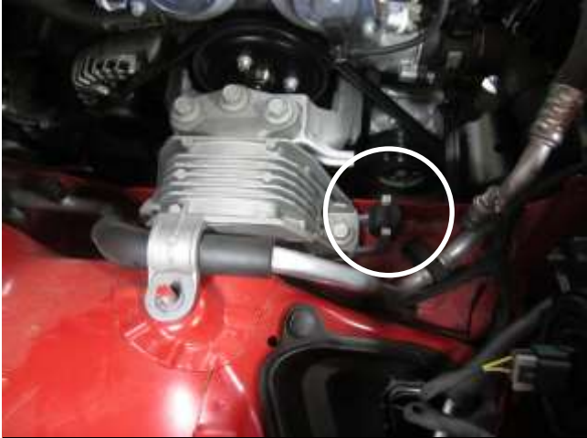
b. Install the rubber grommet that was removed in step 2f. into the mount location as shown.
