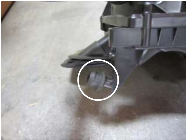
f. Remove the rubber grommet from the stock air box. This will be reused in step 3b.
