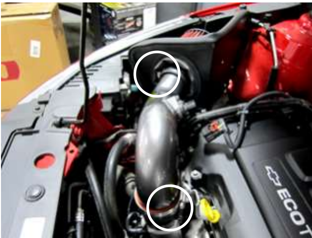
k. Once proper alignment is achieved, tighten all of the hose clamps at the filter and the turbo air inlet.
