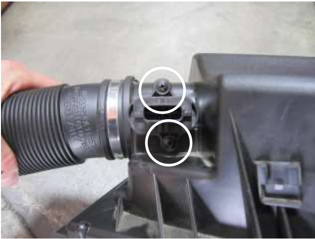
e. Remove the two screws securing the mass air sensor to the air box. Note: The screws will not be reused. The sensor will be reused in step 3h.
