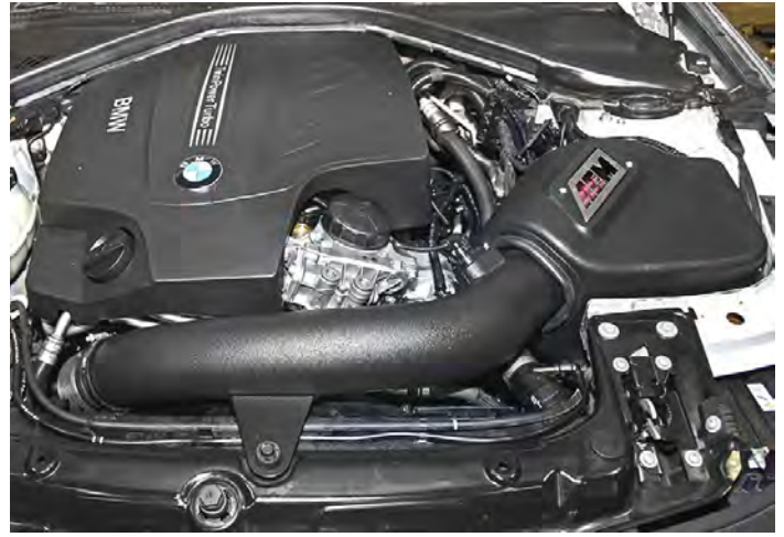
AEM INTAKE INSTALLED
