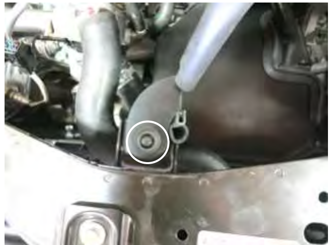
h. Seat the grommet onto the air box post as shown. Note: On 2022 and later models it will be necessary to secure the heat shield with the factory air box mounting bolt.
