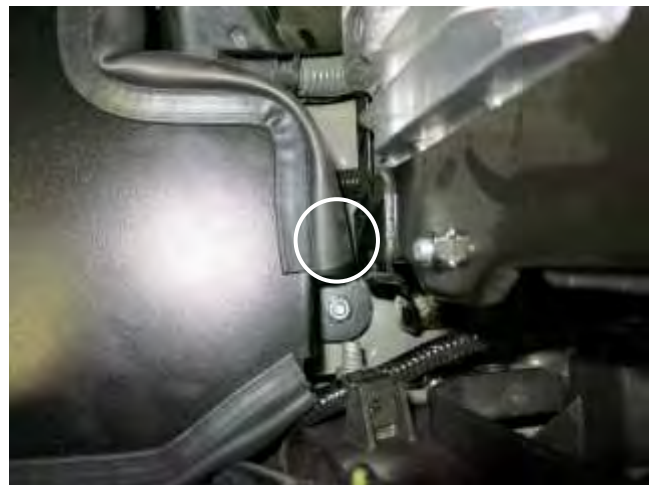
j. With the provided hardware, secure the AEM heat shield to the previously installed rubber mount on the frame rail.
