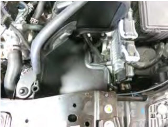
g. Install the AEM heat shield into the vehicle as shown, routing it around the electrical harness.
