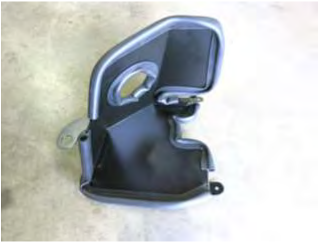
e. Install the provided edge trim as shown. Trimming the edge trim will be necessary.
