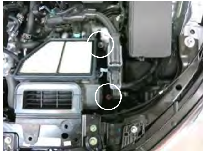
h. Remove the two bolts that secure the lower air box to the vehicle.
