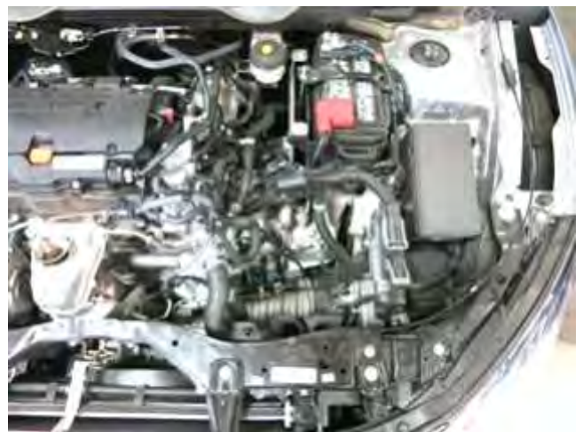
j. Lower air box removed.
