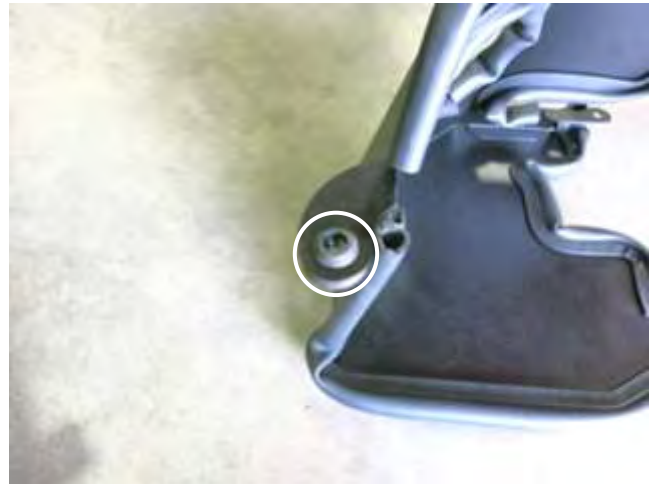
f. Install the grommet that was removed in step 2k. as shown.
