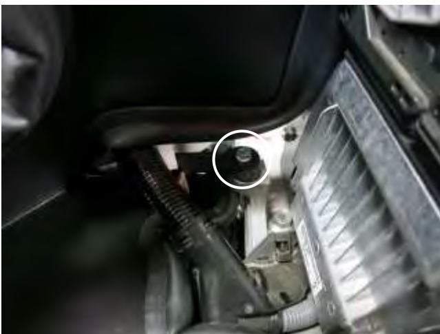
i. With the provided hardware, secure the AEM heat shield to the previously installed rubber mount towards the rear of the vehicle.
