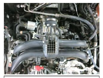
a. Install the hose coupler and 2 hose clamps onto the throttle body. Tighten clamp on the throttle body.
