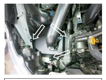
g. Align the heat shield for proper fitment, then secure with 3 supplied M6 bolts. Then, tighten the clamp in 3f.
