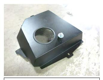
c. Install the edge trim and rubber mount to the heat shield as shown.
