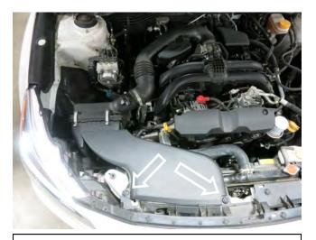
b. Remove the 2 clips that secure the intake scoop.
