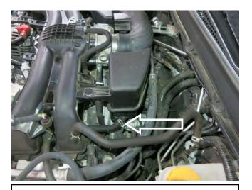
e. Remove the vent hose from the resonator nipple by using pliers to relieve pressure on the hose clamp.
