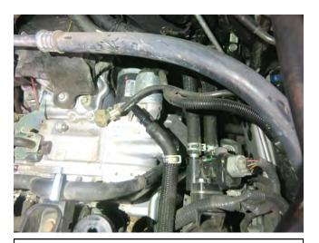
h. Install the plastic connector to the vent hose as shown.
