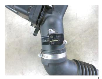
h. Remove the two screws that secure the MAF sensor. Then, set the MAF sensor aside for later installation.
