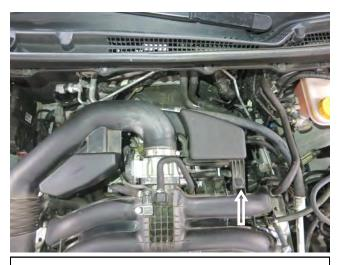
d. Remove the clip that secures the resonator. Also, loosen the hose clamp on the intake tube with an 8mm socket driver.
