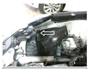
g. Remove the air box bracket bolt with a 10mm socket and ratchet. The bracket will not be reused.
