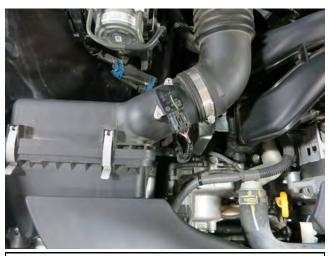
a. Disconnect the plug from the Mass Air Flow (MAF) sensor by pushing on the clip and pull.
