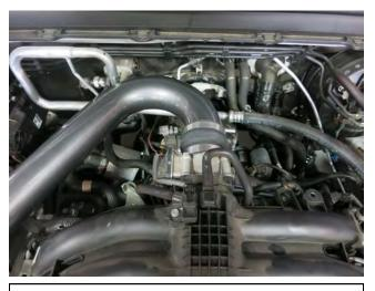
f. Install the AEM intake tube into the coupler. DO NOT FULLY TIGHTEN THE HOSE CLAMP AT THIS TIME.
