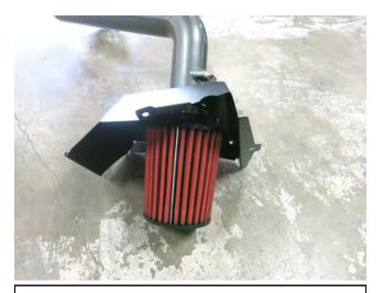
d. Route the intake tube through the cut out on the heat shield and install the air filter.
