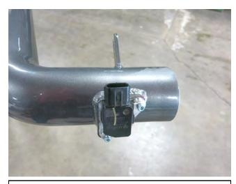
b. Install the MAF sensor to the intake tube with the 2 supplied socket head bolts.
