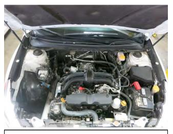
f. Remove the stock intake system from the vehicle. **Do** not discard any factory intake components.
