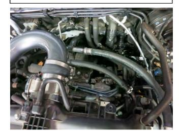
i. Attach the 8" extended hose to the plastic connector then to the intake tube.
