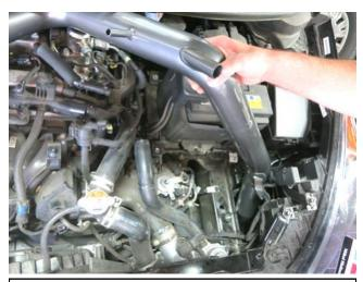
d. Pull the filter end up and over the frame rail to its proper place.
