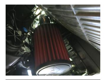
j. Install the filter onto the AEM intake tube, then tighten the band clamp with a 8mm nut driver.
