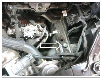
b. Install the 6mm rubber mount in the stock air box mounting hole.
