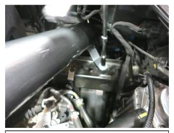
m. Properly align the intake to make sure there is clearance, then tighten the 6mm nut on the rubber mount.
