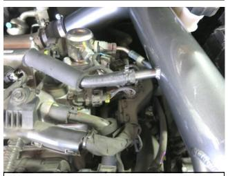
m. Reinstall the PCV hose to the AEM intake tube using the stock spring clamp.
