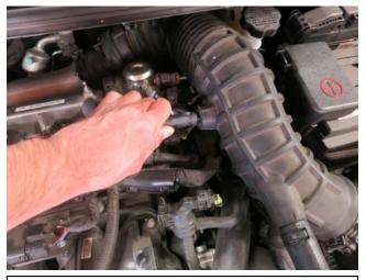
b. Remove the PCV hose from the stock air box tube by using a set of pliers to release the spring clamp.
