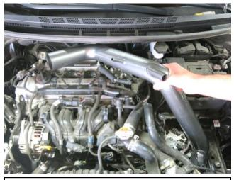
c. Install the AEM intake tube by dropping the filter end inside the frame rail first, then swing the throttle body side in towards the fire wall.
