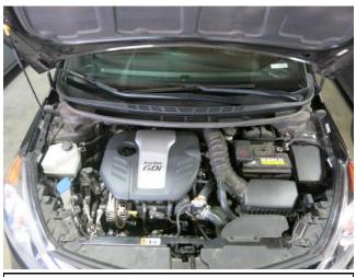
a. Remove the engine cover by lifting up to release it from rubber grommets.
