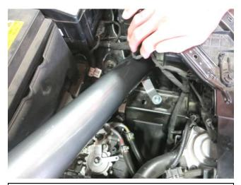
f. Attach the intake tube to the rubber mount. DO NOT TIGHTEN THE BAND CLAMPS UNTIL FILTER IS INSTALLED.
