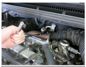
d. Loosen the band clamp with a 10mm socket and ratchet. DO NOT REMOVE INTAKE HOSE UNTIL STEP 2e IS COMPLETED.
