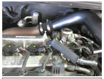
e. Insert the intake tube into the coupler. DO NOT TIGHTEN THE BAND CLAMPS UNTIL FILTER IS INSTALLED.
