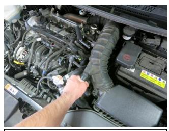
c. Remove the recirculation hose from the stock intake tube by using a set of pliers to release the spring clamp.
