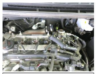
a. Install the coupler and the 2 #44 band clamps.
