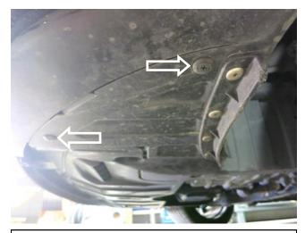
h. Remove the 2 fender liner clips by using a #2 phillips screwdriver.
