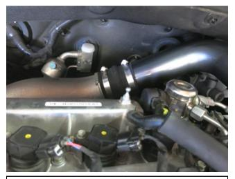
I. Properly align the intake to make sure there is clearance, then tighten the 2 band clamps with an 8mm nut driver. Torque spec: 30in-lb.
