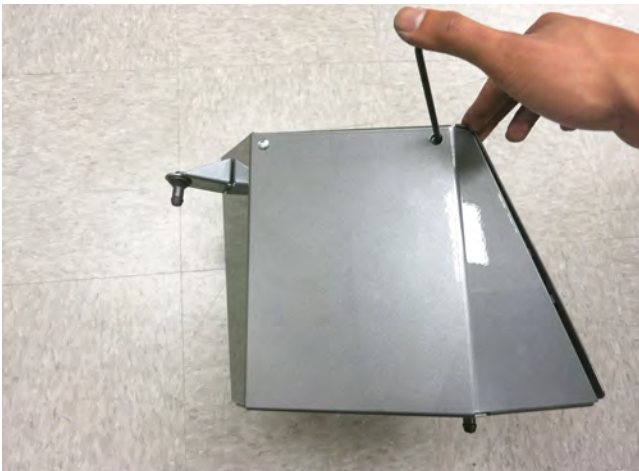
g. Install the two halves of the air box together. Due to variances in the manufacturing process, slight misalignments between the holes and threaded nut-serts may be present. You can align one hole with a small screwdriver while tightening the adjacent hole.
