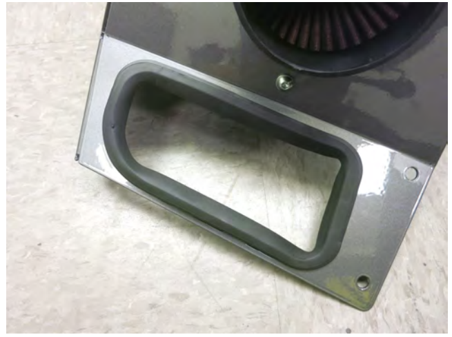
f. Install the rubber gasket removed in step 2g.
