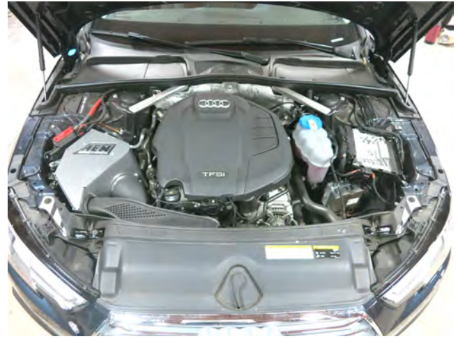
AEM INTAKE INSTALLED
