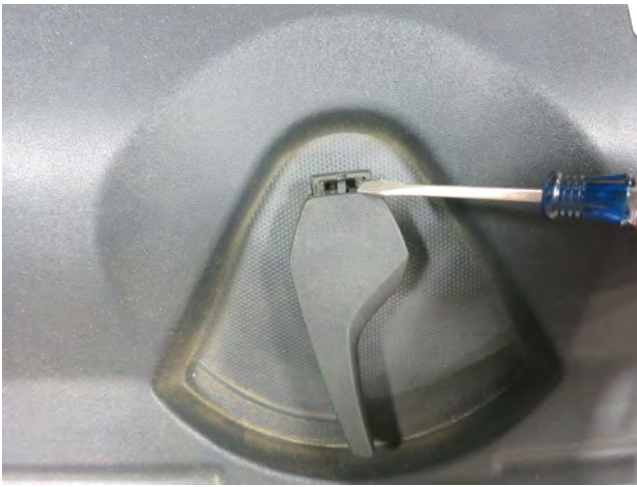
a. Use a small flat head screwdriver to pull out the retaining clip and remove the hood release lever.
