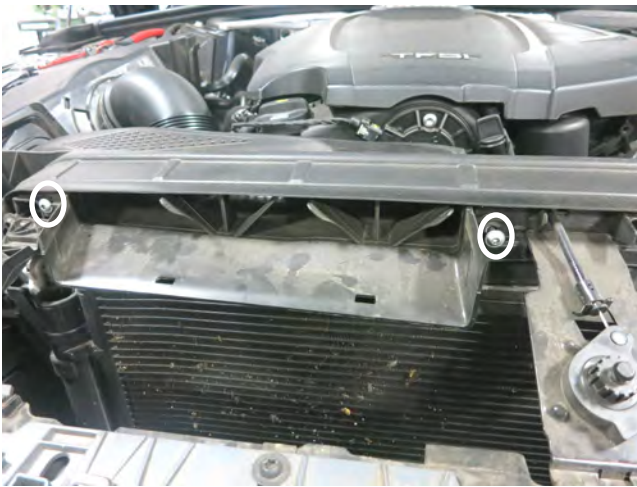
c. Remove the [2] T25 Torx screws shown above and remove the air inlet scoop.
