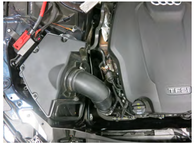
d. Loosen the hose clamp on the intake pipe at the turbo inlet.
