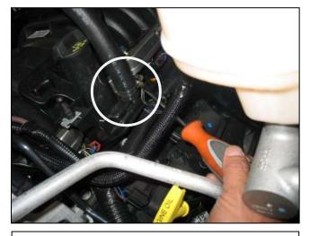
c. With the hose fully engaged on the nipple, fully tighten the hose clamp.
