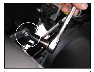
ac. Shift the inlet pipe until the slot in the mounting bracket lines up with the isolator bolt mounted on the heat shield. Place one 8mm flat washer and one M8 nut on the bolt and fully tighten. Now go back and fully tighten the larger air filter and inlet pipe hose clamps.
