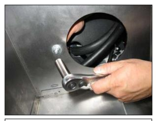
p. Use 1 M8 washer and 1 M8 nut inside the heat shield to secure the rubber mount.
