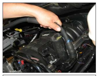
I. Remove the breather tube and hose from the engine.
