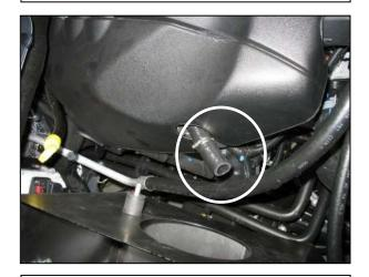
s. Re-install the factory engine cover, allowing the new breather hose to protrude from the access hole as shown. Place the second 1  $\frac{1}{4}$ " hose clamp loosely on the end of the hose.
