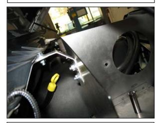
g. Install the rear bracket onto the top lip of the fire wall as shown. Use (Qty. 3) M8 x20mm bolts, (Qty. 3) nuts and (Qty. 6) washers to secure the bracket.
