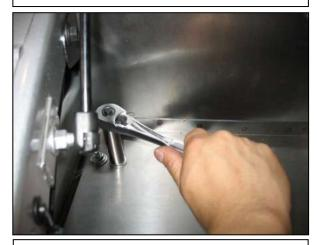
n. Install 2 M8 washers and 2 M8 nuts to secure the bolts positioned in the previous step. Now go back and tighten all the heat shield bracket nuts and bolts installed.
