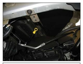
d. Install the bottom heat shield bracket under the passenger side fender rail using the factory bolt removed from Step 2c.
