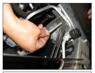
k. Secure the front tab of the bracket to the vehicle using the long bolt removed in step 4i.
