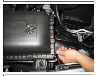
h. Remove the air box lid and inlet duct.
