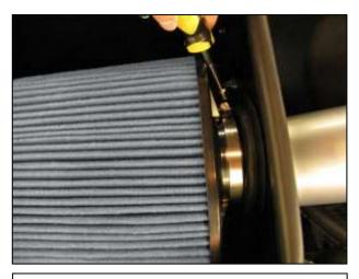
ab. Place the large hose clamp over the air filter's inlet. Place the air filter inside the heat shield and then fully seat the filter onto the filter adapter. Insert the open end of the inlet pipe and loosely secure the hose clamp to hold the air filter in place.
