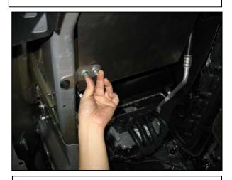
m. At the bottom bracket, hold 2 M8 bolts and 2 washers in position, aligning the bracket to the heat shield.
