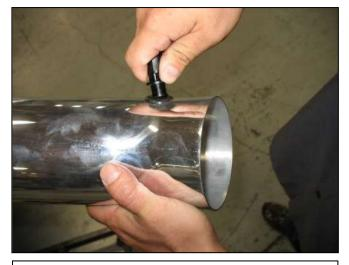
u. Carefully install the IAT sensor into the new inlet pipe using the supplied rubber grommet. If necessary, use soapy water to ease the installation of the grommet; install the IAT sensor into the grommet.
