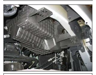
c. With the fender liner removed, access the air box from the bottom of the fender well and remove the 2 bolts securing the air box to the vehicle. Keep the bolts for use in a later step.
