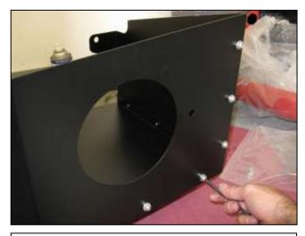
c. Now attach side Panel "B" to both panels "A" and "C" with 9 more M6 button head bolts, lock washers, and flat washers. Install the bolts loosely at first, then tighten them once the panels are in the correct position.
