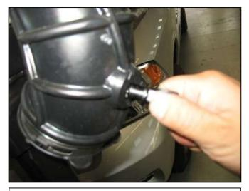
t. Carefully remove the inlet air temperature (IAT) sensor from the OEM inlet duct.
