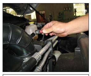
d. Unlock the intake air temperature (IAT) sensor connector by sliding the red tab and pressing the clip to disconnect the wiring harness from the sensor.
