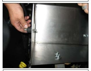
o. Install the rubber isolator mount on the outside of the heat shield assembly as shown.
