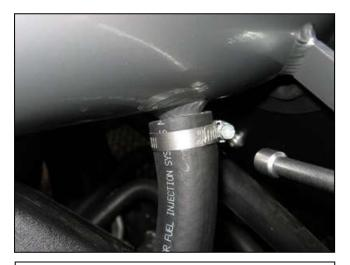
aa. Connect the breather hose to the nipple on the other side of the inlet tube and tighten the 1-1/4" hose clamp.
