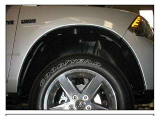
a. Remove all fasteners securing the passenger side fender liner. WARNING:After dropping the liner, be sure to unclip the ABS sensor wiring harness attached to the engine side of the liner.
