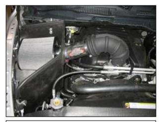
AEM<sup>®</sup> intake system installed
