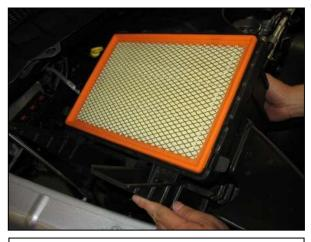
j. Remove the air box base and air filter from the vehicle.
