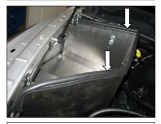
r. Install the short and the long sections of the rubber sponge edge gasket along the top edge of the heat shield as shown.
