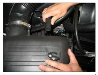
f. Disconnect the engine breather hose from the air box lid.
