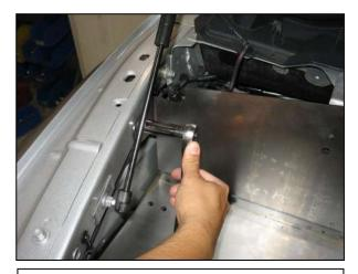
e. Carefully position the heat shield into the vehicle. Use the bolt removed in Step 2i to hold the heat shield in place. Tighten the bolt about <sup>3</sup>/<sub>4</sub> of the way into the thread for now.
