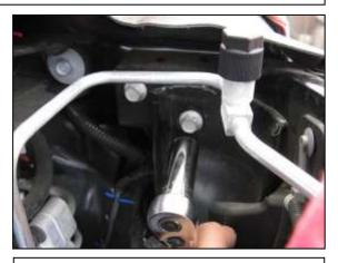
i. On the passenger side of the radiator support, remove the long bolt as shown.
