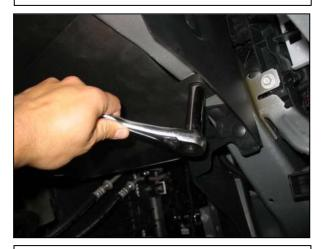
f. On the bottom side of the heat shield, secure the tab coming off the heat shield to the vehicle using the bolt removed in Step 2c. Tighten the bolt about ¾ of the way into the thread for now.
