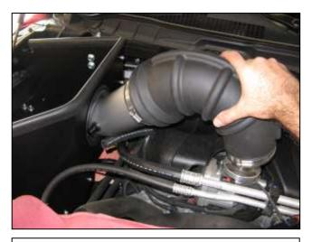
x. Install the intake pipe assembly, inserting the open end through the large hole in the heat shield while also mounting the elbow inlet onto the throttle body neck.
