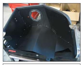
d. Here is the complete heat shield assembly. You may install the sponge rubber gaskets in the large hole (medium length gasket) and along the top edges (short and long gaskets) as shown at this time. Trim any excess as needed.
