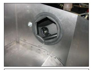
q. Install the medium section of the rubber sponge edge gasket in the large hole for the inlet tube as shown.
