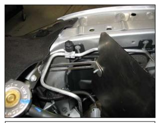
j. Install the front bracket to the heat shield using an M8 x 20mm bolt, a nut, and 2 washers. The bracket has 2 bent tabs at its ends. Make sure the longer tab mates to the heat shield.
