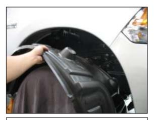
b. Remove the fender liner from the vehicle.
