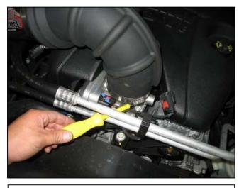
y. Tighten the smaller hose clamp of the elbow inlet at the throttle body.
