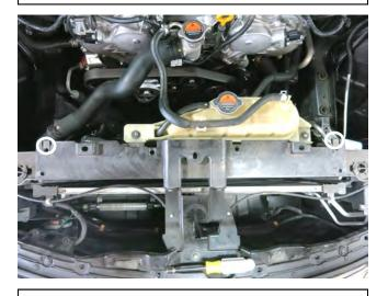
d. Install the [2] clip nuts onto the upper core support in the locations shown above.
