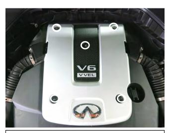
b. Use a 10mm socket and ratchet to remove the [2] nuts and [3] bolts holding the engine cover. Remove the
