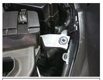
d. Remove the M6 bolt in the location shown above.
