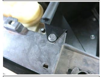
i. Secure the front of the heat shield with the supplied M6 bolt. Repeat for other side.
