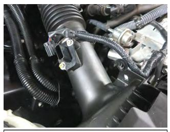
c. Unplug the Mass Air Flow (MAF) sensor harness and unclip it from the air box. Repeat for other side.
