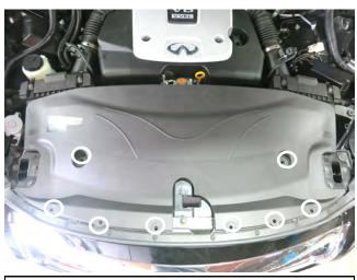
a. Use a small flat head screwdriver to remove the [8] clips holding the radiator shroud. Remove the shroud.
