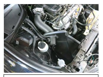
g. Install the intake tube with heat shield into the vehicle. Insert the intake tube into the coupler. Install the breather hose onto its respective port. Then fully seat the post mounts on the heat shield into the grommets on the frame rails.
