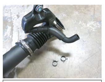
k. Remove the [2] spring clamps from the breather hose (passenger side pictured). Do not discard any factory components or hardware removed thus far.
