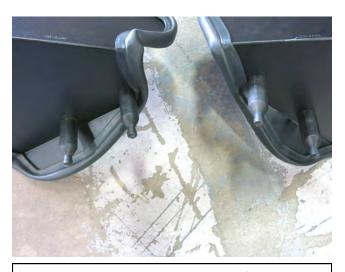
f. Install the post mounts to the bottom of the heat shields.
