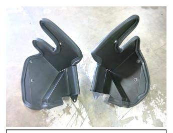
e. Apply the supplied edge trims to the heat shields as shown above. Trim if needed.
