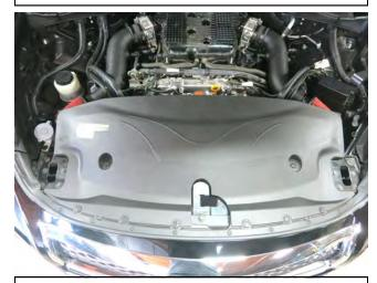
n. Reinstall the radiator shroud and engine cover.
