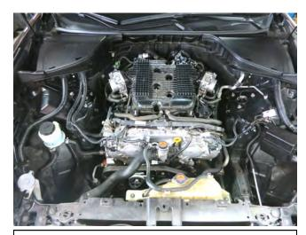
h. Loosen both throttle body hose clamps and the pull both intake tubes and air boxes from the engine bay. Make sure the [4] grommets are still seated in the frame rails.
