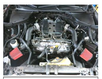
I. Install the AEM filters. Orient them for best fit. Then tighten the hose clamps on the throttle body couplers to fully secure the intake tubes.
