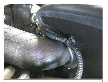
m. Route the MAF harness above the intake tube and clip it into the provision on the heat shield. Repeat for other side.
