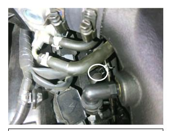
j. Reposition the spring clamp onto the breather hose (driver side pictured).
