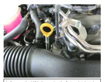
d. Remove the M6 bolt securing the factory intake tube.
