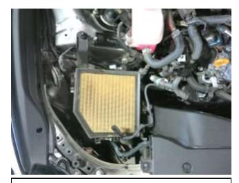
f. Undo the [4] airbox latches and remove the upper intake assembly.
