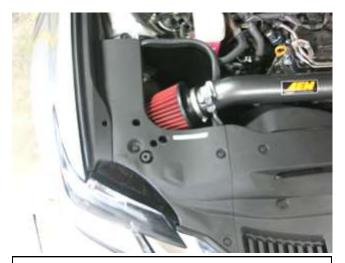
m. Reinstall the plastic shroud with the [4] retention clips. To reinstall the retention clips: Pull the mandrel from the main clip, insert the clip into its respective location, and reinsert the mandrel.
