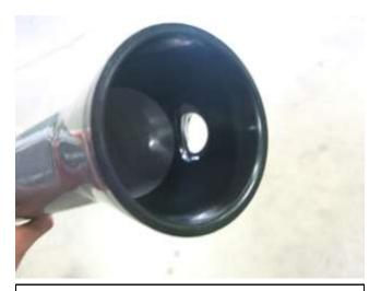
b. Insert the venturi into the intake tube. Be sure to align the pass-thru cutout in the venturi with the hole for the MAF sensor on the AEM intake tube.
