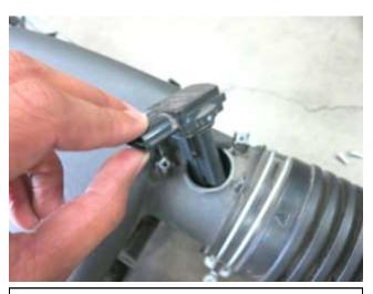
k. Remove the MAF sensor from the factory intake tube. Do no discard any factory components or hardware removed thus far.
