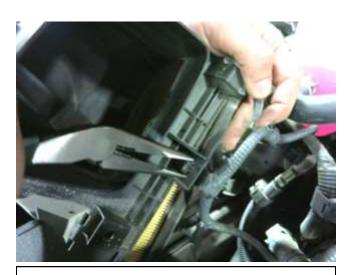
h. Flip the lower airbox around and unclip the MAF harness.
