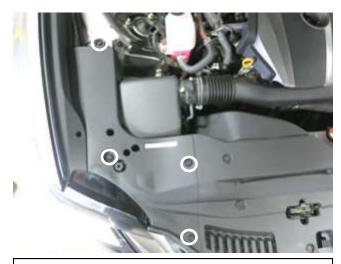
b. Remove the [4] retention clips by depressing the mandrel in the center. Then pull off the plastic shroud.
