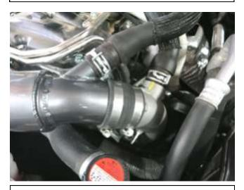
i. Insert the AEM intake tube into the turbo inlet coupler. Leave the hose clamp loose. Connect the PCV hose to the port on the intake tube.
