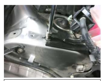
j. Remove the M6 bolt securing the ground cable bracket.
