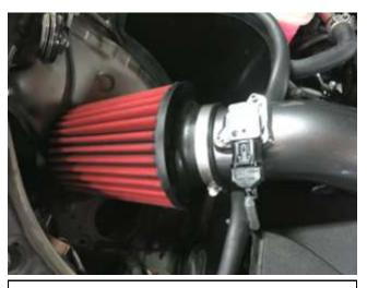
I. Install the AEM filter and tighten the hose clamp on the filter.
