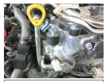
e. Install the rubber mount, washer, and nut onto the bracket as shown. Leave the nut loose.
