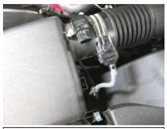
c. Unplug the Mass Air Flow (MAF) sensor harness and unclip it from the upper air box.
