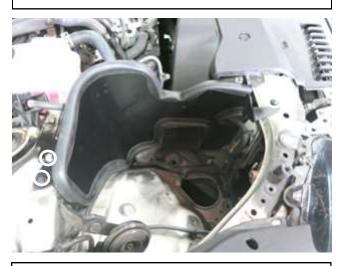
g. Place the heat shield into the engine bay. Make sure the cold air scoop is properly aligned in the heat shield cut-out. Then secure with the supplied M6 bolt and the [2] M6 bolts removed in steps 2i & 2j.
