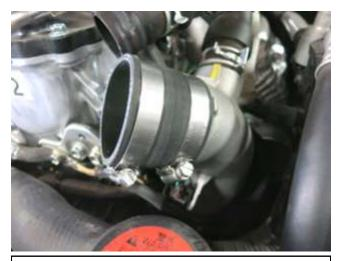
d. Install the coupler with hose clamps onto the turbo inlet pipe. Make sure the smaller end of the coupler is fitted to the turbo inlet side. Tighten the hose clamp on the turbo inlet side at this time.
