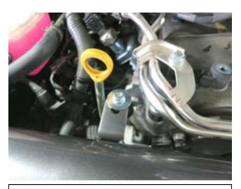
j. Align the mounting bracket to the rubber mount. Position the tube for best fit, then tighten the nut. Also, tighten, the hose clamp left loose in previous step.
