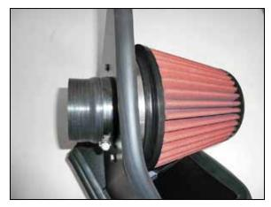
10. Install the provided air filter and coupling hose (5-352) onto the filter adapter and secure with the provided hose clamps.
