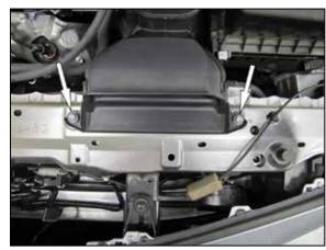
3. Remove the two bolts that secure the fresh air intake duct and then remove the duct from the vehicle.
