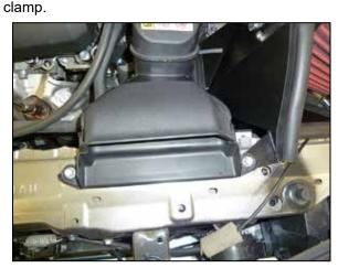
13. Install the fresh air intake duct and secure with the factory hardware.
