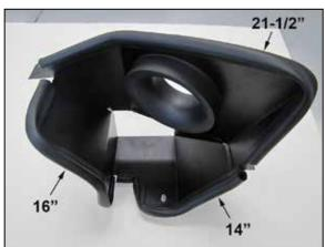
8. Cut the provided top bulb edge trim into sections of 21-1/2", 16" and 14" and then install them onto the heat shield as shown.
