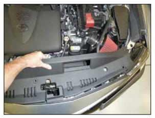
14. Reinstall the radiator cover and secure with the factory push clips.
