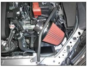
11. Install the heat shield assembly into the vehicle so the mounting studs engage the factory mounting grommets.
