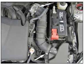
5. Loosen the hose clamps that secure the intake tube to the throttle body and air filter housing, unhook the vent lines attached to the intake tube and then remove the tube from the vehicle.
