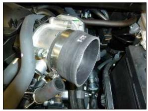
12. Install the provided coupler hose (5-326) onto the throttle body and secure with the provided hose
