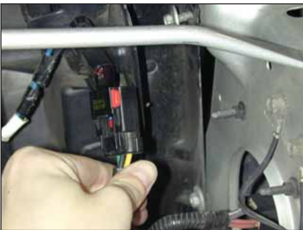
d. Unplug the fan wiring harness from the fan.
