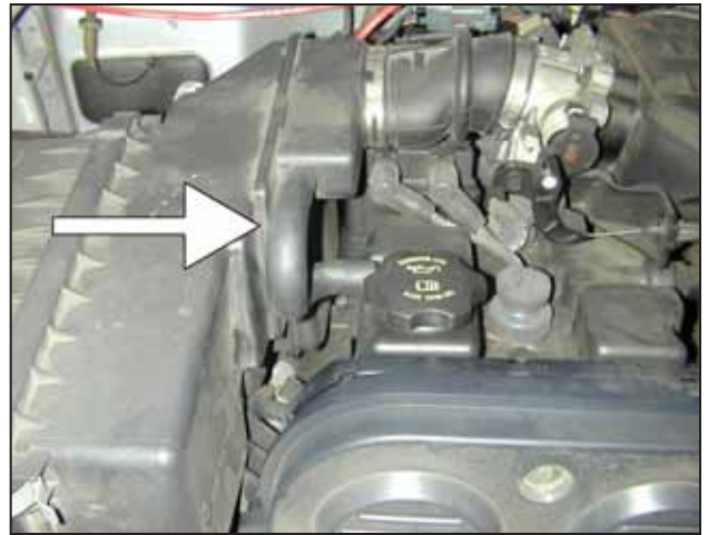
b. Disconnect the breather hose from the air filter housing.
