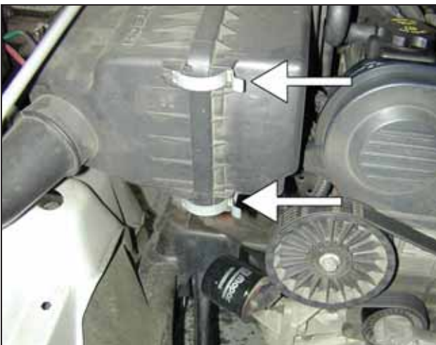
c. Unclip the two metal retaining clips on the air filter housing. Remove the air filter housing lid and air filter.
