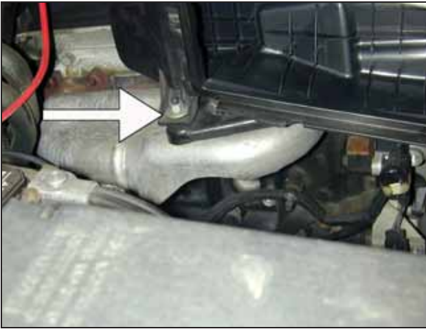
e. Remove the nut securing the air filter housing to the engine.
