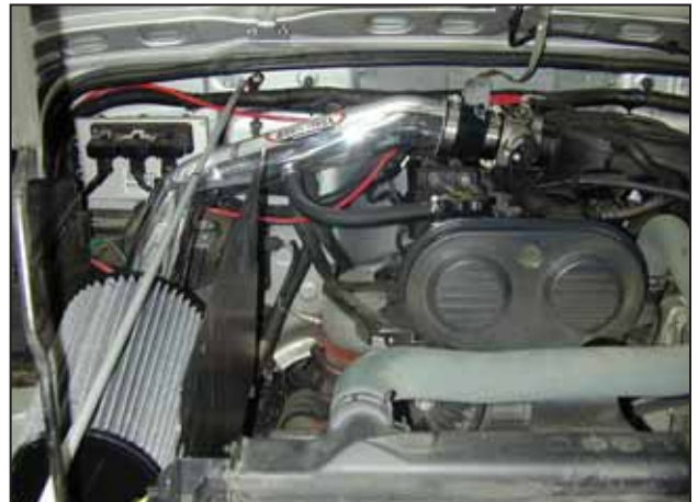
AEM® intake system installed
