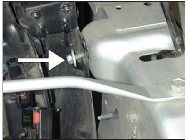
c. Remove the bolt on the passenger side radiator support as shown.
