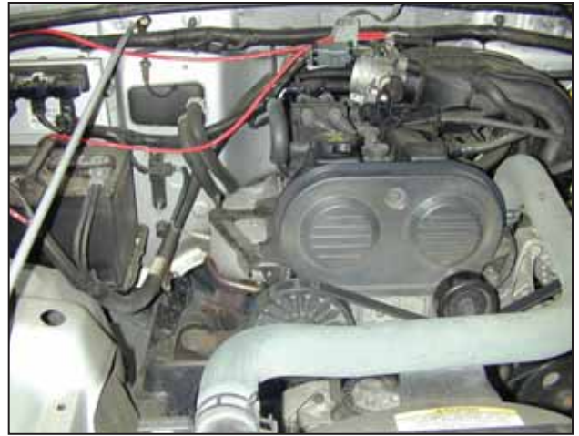
f. Remove the air filter housing from the engine compartment.
