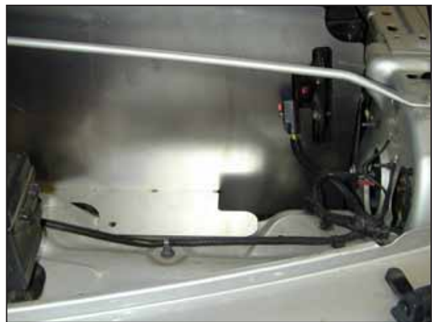
e. Install the heat shield into the engine compartment and align the front mounting tab with the bolt removed in step 3c.
