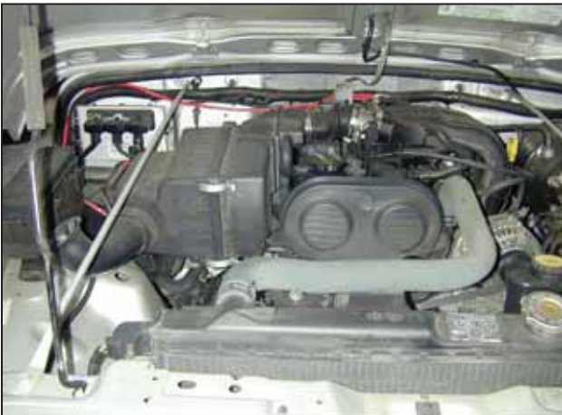
Factory air box system installed
