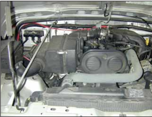
a. Factory air box system installed.
