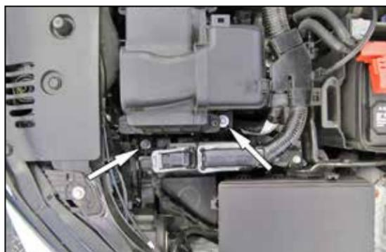
4. Remove the two bolts that secure the air filter housing to the vehicle.
