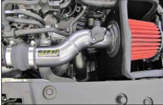
11. Install the AEM® intake tube through the heat shield and into the AEM® air filter, then install onto the turbo inlet. Align the tube for best fit and then secure with the provided hose clamp.
