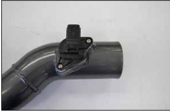
10. Remove the mass air sensor from the factory air filter housing and install it into the AEM® intake tube and secure with the provided hardware.
