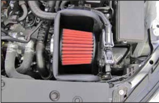
8. Set the AEM® air filter into the heat shield assembly.
