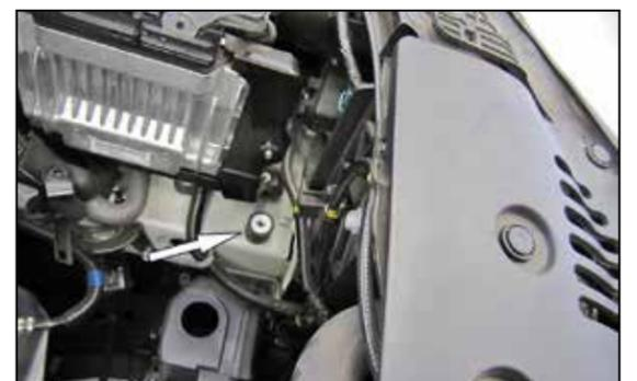
5. Install the rubber mounted stud onto the frame rail where shown.
