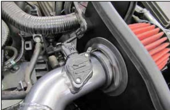
12. Reconnect the mass air sensor electrical connection.
