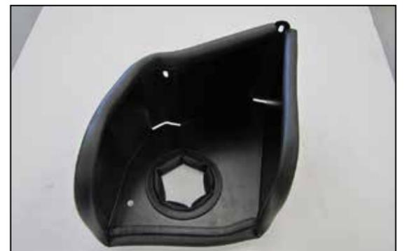
6. Install the provided edge trim onto the heat shield as shown.
