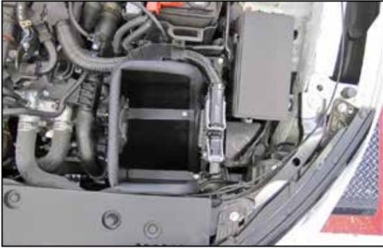
7. Install the heat shield assembly onto the frame rail and secure with the provided hardware.
