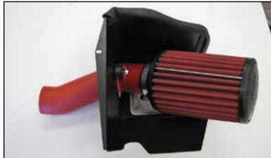
11. Install the AEM® air filter onto the intake tube and secure with the provided hose clamp.
