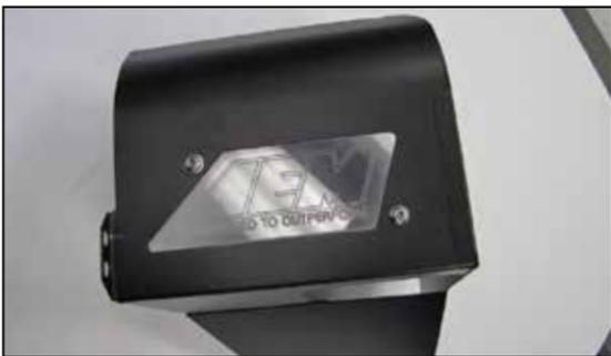
7. Install the AEM® window into the heat shield using the provided hardware and backing plate.
