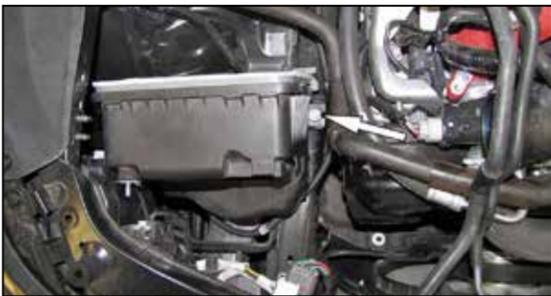
6. Remove the bolt that secures the dirty side air filter housing to the frame rail and then remove the air filter housing from the vehicle.
