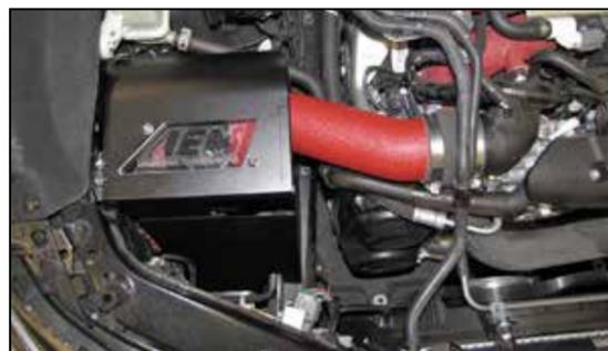
13. Install the intake assembly into position, be sure to connect the mass air sensor electrical connection. Insert the intake tube into the coupler at the turbo inlet tube. Adjust the assembly for best fit and then secure with the provided hardware.
