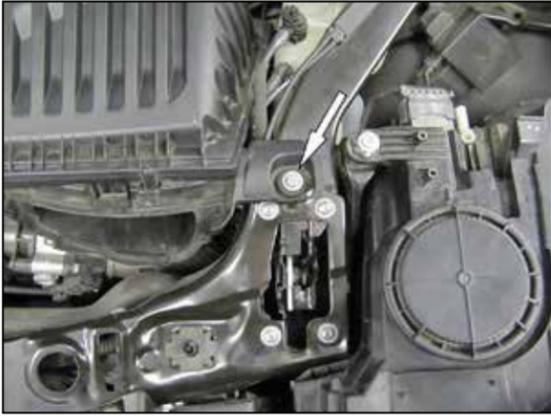
4. Remove the bolt that secures air filter housing to the core support.
