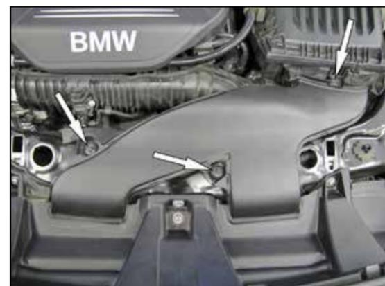
3. Remove the two bolts that secure the fresh air intake duct too the core support. Release the locking tab at the air filter housing and then remove the fresh air intake duct.
