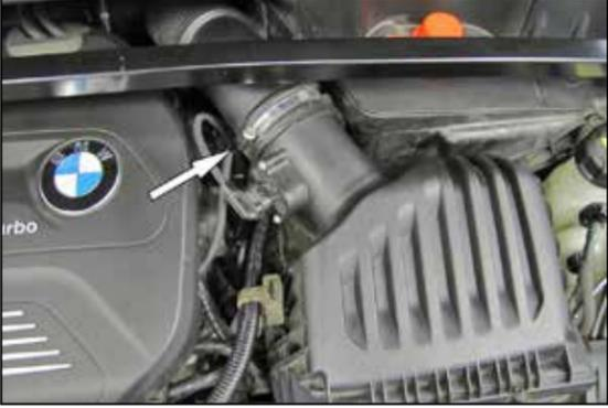
5. Loosen the hose clamp that secures the intake hose to the air filter housing then remove the air filter housing from the vehicle.
