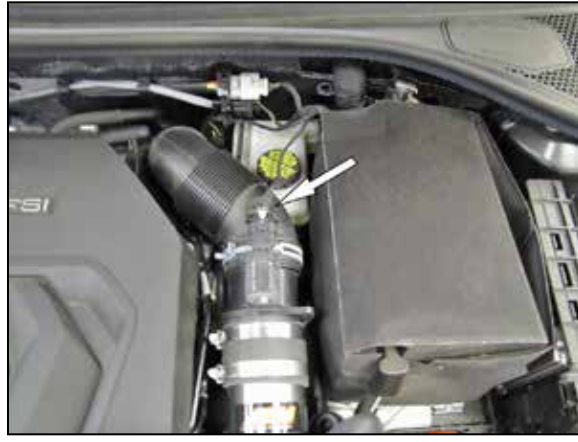
20. Reconnect the mass air sensor electrical connection.
