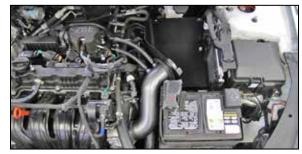
11.Install the AEM<sup>®</sup> intake tube into the heat shield and into the coupler at the throttle body, adjust the tube for best fit and then secure with the provided hose clamp.
