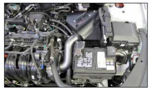
14. Install the cover onto the heat shield and secure with the provided hardware.
