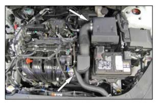
4. Loosen the hose clamps that secure the factory intake tube and then remove the intake tube from the vehicle.
