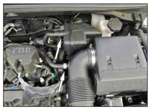
3. Disconnect the breather hoses from the factory intake tube and intake plenum.
