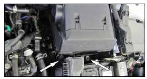
5. Remove the two bolts that secure the factory air filter housing and then remove the factory housing from the vehicle.
