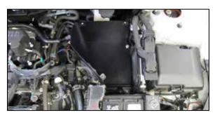
9. Install the heat shield into the vehicle so the mounting stud inserts into the mounting grommet and it aligns with the rubber mounted studs, then secure with the provided hardware.
