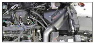
15. Connect the factory vent lines to the lines installed onto the AEM<sup>®</sup> intake tube.
