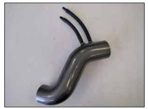
10. Install the provided vent lines and fittings onto the  $AEM^{\circledast}$  intake tube as shown.
