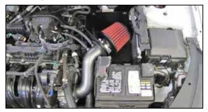
12. Install the AEM<sup>®</sup> air filter onto the intake tube and secure with the provided hose clamp.
