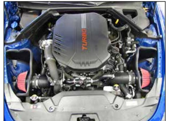
20. Install the provided AEM® air filters onto the filter adapters and secure with the provided hose clamps.
