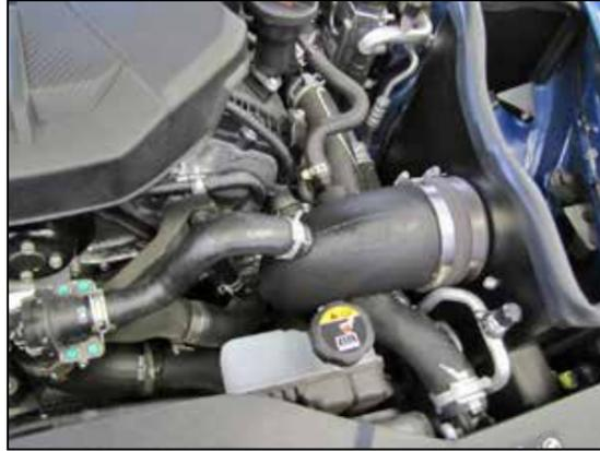
13. Install the provided filter adapter into the heat shield so that it goes through the heat shield and into the coupler on the intake tube. Secure the adapter to the heat shield using the provided hardware and then adjust the intake tube and couplers for best fit and secure with the provided hose clamps. Connect the vent lines to the fittings in the intake tube and install the factory passenger BOV hose and secure with the factory clamps.
