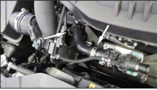
7. Release the spring clamps that secure the passenger side BOV hose to the BOV and intake tube, then remove the Passenger side BOV hose.
