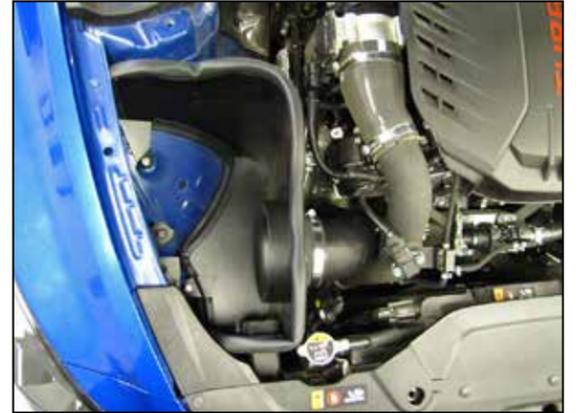
18. Install the provided filter adapter into the heat shield so that it goes through the heat shield and into the coupler on the intake tube. Secure the adapter to the heat shield using the provided hardware and then adjust the intake tube and couplers for best fit and secure with the provided hose clamps.
