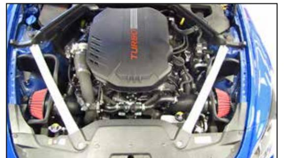
21. Reinstall both strut tower braces and secure with the factory hardware.
