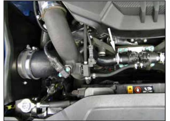
19. Install the driver's side BOV hose and secure with the factory hose clamps.
