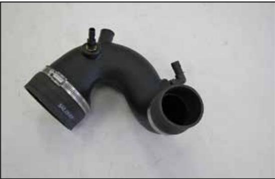
10. Install the provided couplers (5-222N & 08761) onto the Drivers side intake tube (9-0459) and then install the 90° and straight vent fittings as shown.
