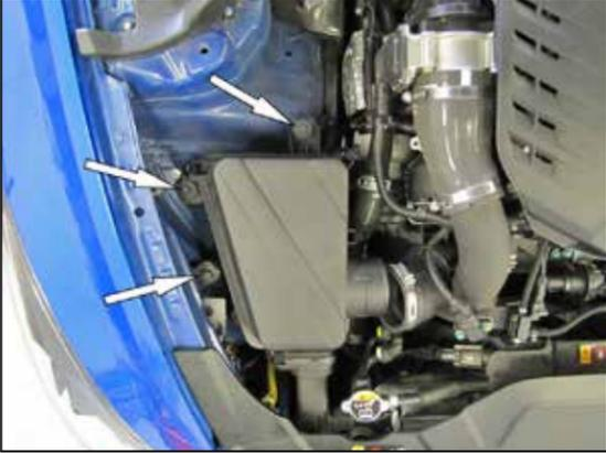
8. Remove the three bolts that secure the passenger side air filter housing to the inner fender, loosen the hose clamp that secures the intake tube to the air filter housing and disconnect the tube. Remove the passenger side air housing from the vehicle.
