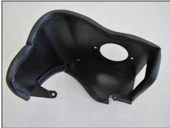
14. Trim and install the edge trim 35", 16" and 2-1/2" onto the passenger side heat shield (20-8634) as shown.
