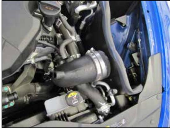
12. Install the driver's side heat shield assembly into the vehicle and secure with the provided hardware. Then install the intake tube assembly onto the turbo inlet.
