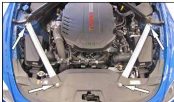
2. Remove the four bolts shown that secure the two strut tower braces to the vehicle and then remove the braces from the vehicle.
