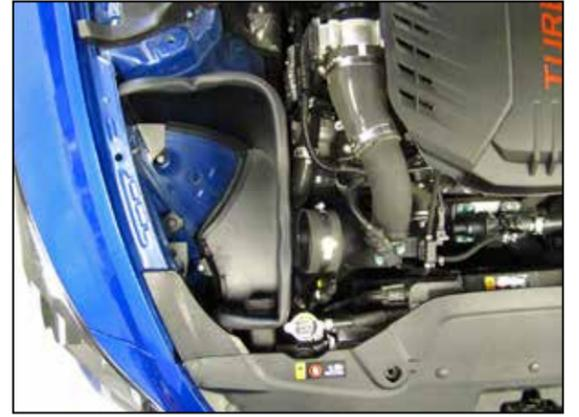
17. Install the passenger side heat shield and secure with the provided hardware.
