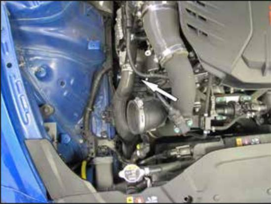
9. Loosen the hose clamp that secures the intake tube to the passenger side turbo and then remove the intake tube from the vehicle.
