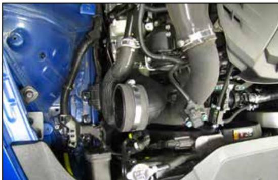
16. Install the passenger side intake tube onto the turbo inlet.
