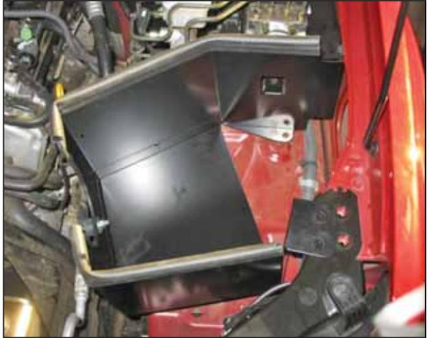
c. Insert the heat shield into the engine bay.
