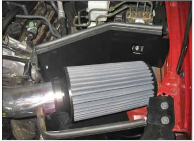
m. Attach the air filter and secure to the intake pipe. Check for clearance around the air filter.
