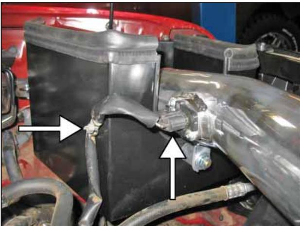
j. Plug in the MAF sensor harness into the MAF sensor. Secure the MAF sensor wire harness to the heat shield as shown.
