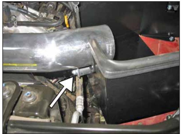
i. Secure the bracket to the rubber mount with the provided washer and nut.
