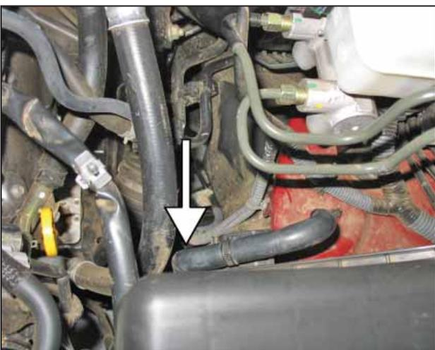
i. Remove the transmission breather hose from the air box.
