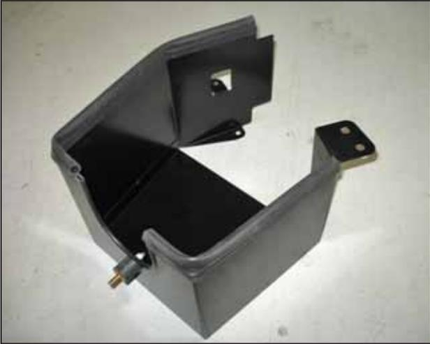
b. Install the rubber mount on the heat shield, using the supplied washer and nut. Install the rubber edge trim (#8-3010) around the intake pipe opening. Also install the edge trim (#8-4017) on the top edges of the heat shield.
