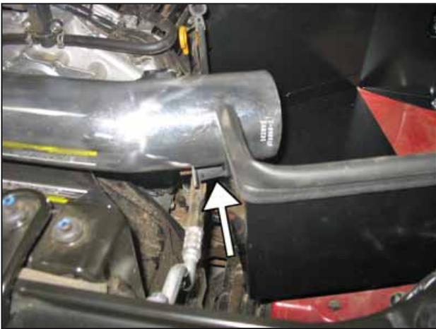
h. Line up the intake pipe's bracket with the rubber mount installed on the heat shield. Ensure the intake pipe has proper clearance, then secure the hose clamp at the throttle body.
