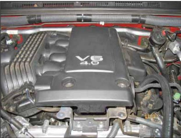
n. **2WD Vehicles:** Reinstall the engine cover and proceed to section 4.
