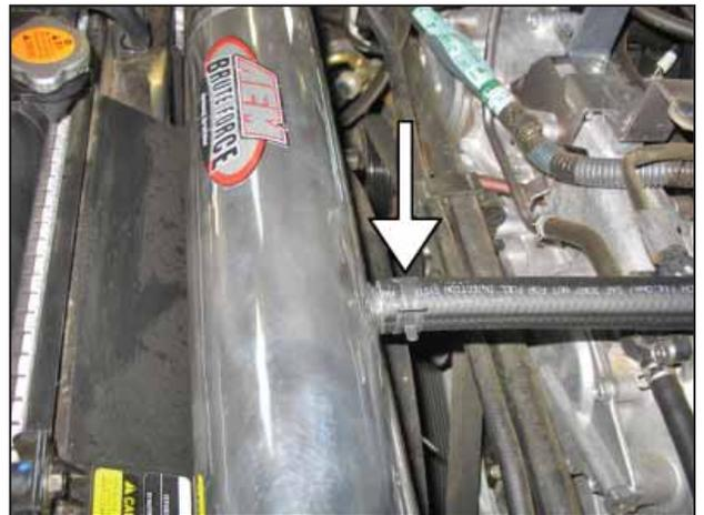
k. Attach the crank case breather hose to the intake pipe and secure with the factory spring clamp.
