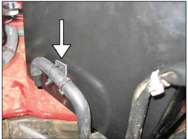
o. Secure the transmission breather hose to the heat shield with the zip tie and mount as shown.
