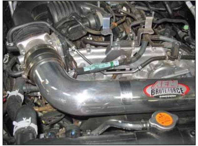
g. Insert the intake pipe into the coupler, secure in place, but do not completely tighten the hose clamps.
