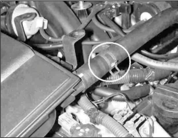
e. Unclasp the spring clamp and remove the breather hose from the air inlet tube. Save the spring clamp for later use.
