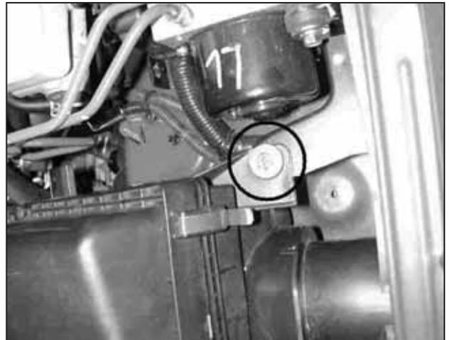
h. Remove the rear mounting bolt to the air box. Remove the air box from the engine bay.
