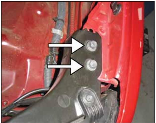
e. Secure the tab at the radiator support with the stock bolts as shown.
