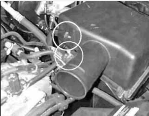
g. Unplug the MAF sensor and remove the MAF sensor harness.
