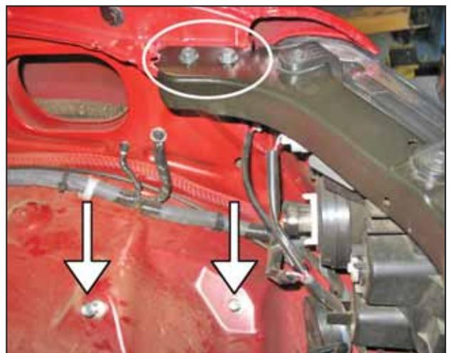
j. Remove the air box mounting bolts. Also remove the two bolts from the radiator support.
