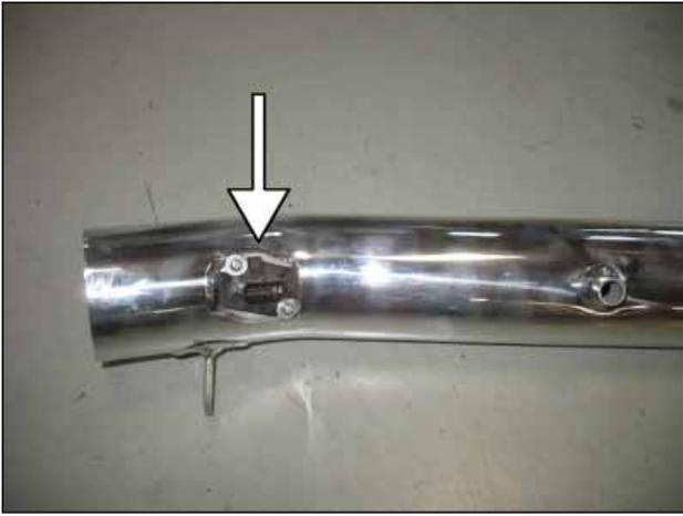
f. Insert the MAF sensor and secure with the factory hardware as shown.
