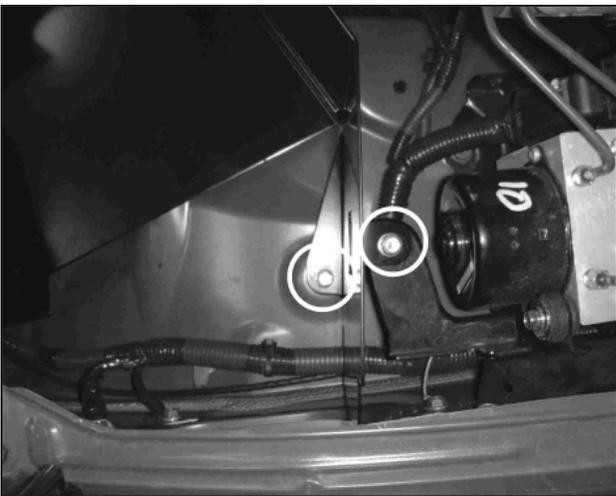
d. Secure the heat shield on both tabs as shown.
