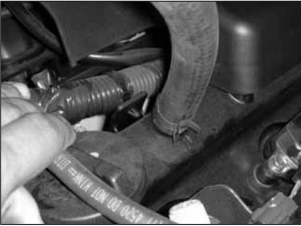
l. Attach and secure the other end of the breather hose to the crank case vent, secure with the factory hose clamp.
