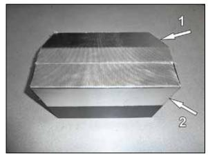
10. Install the provided heat shield insulation strips onto the bottom of the heat shield as shown. Some trimming of the insulation strips excess will be necessary.
