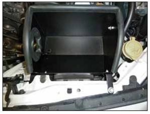
16. Set the heat shield into position on the core support and secure with the factory air box mounting bolts and to the previously installed bracket with the hardware provided.
