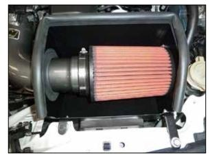
22. Install the air filter onto the AEM<sup>®</sup> intake tube and secure with the provided hose clamp.
