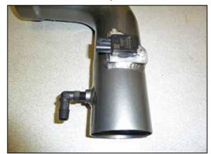
17. Remove the mass air sensor from the factory air filter housing and then install it into the AEM®
