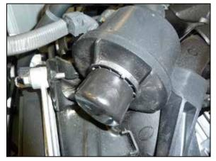
21. Install the provided caplug onto the sound drum.
