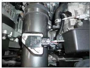
20. Connect the crank case vent to the fitting installed into the AEM<sup>®</sup> intake tube as shown. Reconnect the mass air sensor electrical connection.
