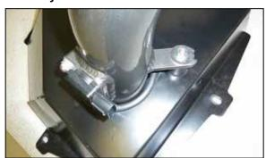
11. Install the intake tube into the heat shield as shown and secure it to the rubber mounted stud with the provided hardware.
