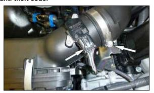
2. Disconnect the mass air sensor electrical connection. Loosen the hose clamp that secures the air filter housing to the intake tube.
