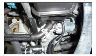
6. Release the spring clamp that secures the vent line to the intake resonator then disconnect the vent line from the resonator. Remove the factory intake tube from the vehicle.
