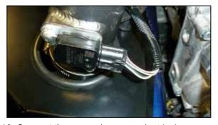
16. Connect the mass air sensor electrical connection.
