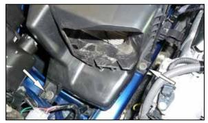
4. Remove the two bolts that secure the factory air filter housing to the inner fender then pull the air filter housing up to unlock it from the mounting grommet and remove it from the vehicle.
