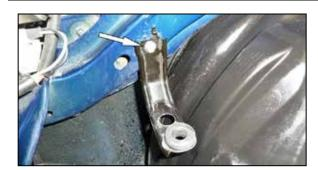
7. Remove the factory air filter housing mounting bracket from the inner fender.
