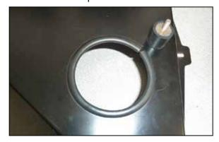
10. Install the provided edge trim into the hole of the heat shield that the intake tube will pass through. Install the provided rubber mounted stud onto the heat shield and secure with the provided hardware.
