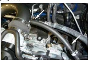
15. Install the provided crank case vent hose onto the fitting installed in the previous step and then connect the open end to the AEM® intake tube as shown.
