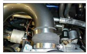
13. Install the intake tube into the coupler at the throttle body and position the heat shield onto the inner fender. Adjust the intake system for best fit and then secure with the provided hose clamp and
