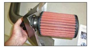
12. Install the AEM® air filter onto the intake tube and secure with the provided hose clamp.
