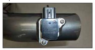
9. Remove the mass air sensor from the factory air filter housing and install it into the AEM® intake tube and secure with the provided hardware.
