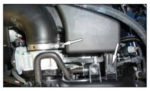
5. Remove the clip that secures the intake resonator to the engine then loosen the hose clamp that secures the intake tube to the throttle body.
