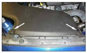
3. Remove the two retaining clips that secure the fresh air intake duct and then remove the intake duct from the vehicle.
