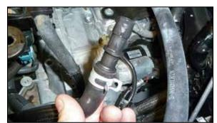
14. Install the provided union fitting into the factory crank case vent fitting and secure with the factory
