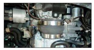
8. Install the provided hump coupler onto the throttle body and secure with the provided hose clamp.
