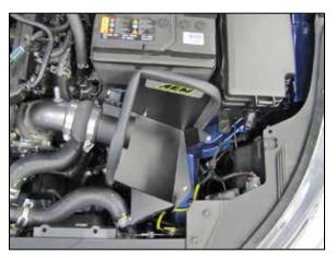
10. Install the heat shield and secure with the provided hardware. Install the AEM<sup>®</sup> intake tube into the couplers and adjust for best fit and secure with the provided hose clamps.
