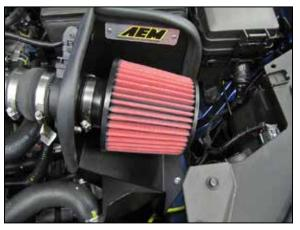
12. Install the AEM<sup>®</sup> air filter and secure with the provided hose clamp.
