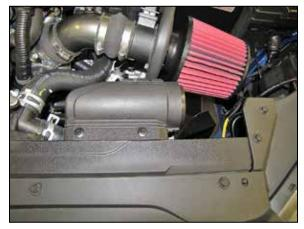
13. Remove the hose from the fresh air intake duct and then reinstall the duct and secure with the factory retaining pins.
