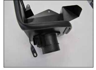
8. Remove the mass air sensor from the factory air filter housing and install it into the AEM<sup>®</sup> heat shield and secure with the provided hardware. NOTE: Remove the O-ring seal from the mass air sensor housing before installing it onto the heat shield.
