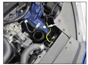
4. Install the rubber mounted stud into the frame rail at the air filter housing mounting location.
