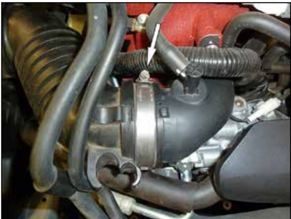
4. Loosen the hose clamp that secures the intake hose to the turbo inlet.
