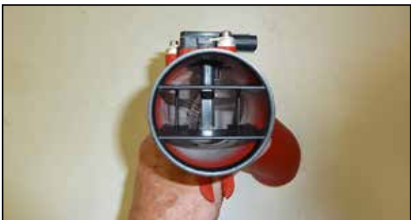
13. Place three small drops of the provided glue next to the lip of the maf sleeve and then install the maf sleeve so that the blades are perpendicular to the maf as shown.
