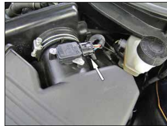
3. Disconnect the mass air sensor electrical connection.
