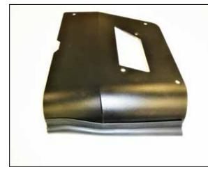
19. Install the remaining edge trim onto the heat shield lid as shown.
