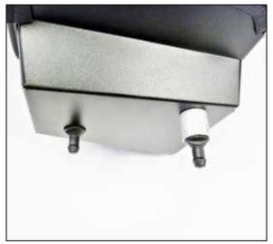
11. Install the heat shield mounting studs onto the heat shield using the provided hardware and spacer.
