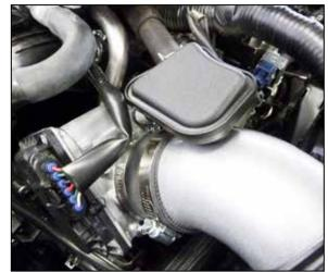
7. Remove the bolt shown that secures the lower air filter housing to the core support.
