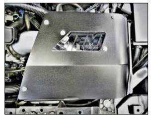
21. Install the lid onto the heat shield and secure with the provided hardware.
