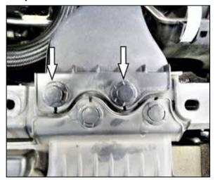
6. Remove the two plastic retaining clips that secure the fresh air intake duct.
