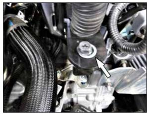
8. Remove the bolt that secures the wiring harness.
