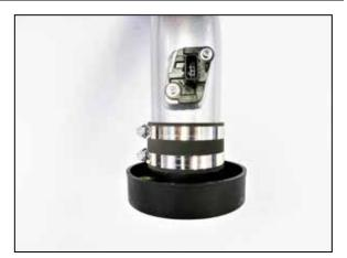
14. Remove the mass air sensor from the factory air filter housing and install it into the AEM intake tube using the provided hardware. Using the provided coupler, Install the filter adapter onto the AEM intake tube as shown.
