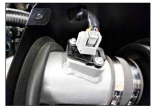
18. Pass the mass air sensor harness through the hole in the heat shield and then reconnect the mass air sensor electrical connection.
