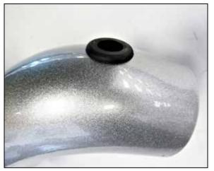
13. Install the provided grommet into intake tube as shown.
