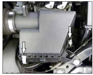
5. Release the two retaining clips that secure the upper air filter housing to the lower air filter housing. Remove the upper air filter housing and factory air filter.
