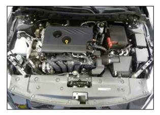
2. Remove the twelve plastic retaining clips that secure the upper valence and then remove the valence from the vehicle.
