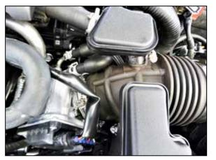
4. Disconnect the CCV hose and chamber from the factory intake tube. Loosen the hose clamp that secures the intake tube to the throttle body.
