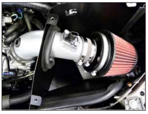
16. Install the tube assembly through the heat shield and then into the coupler at the throttle body, adjust the tube for best fit and then secure the hose clamp.
