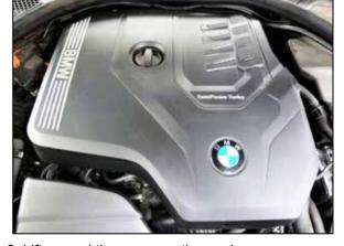
2. Lift up and then remove the engine cover.
