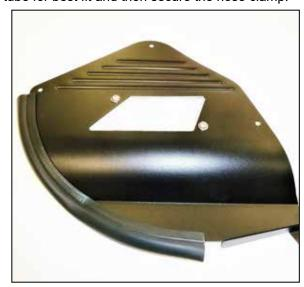
15. Install the AEM window into the lid and then install the edge trim as shown.
