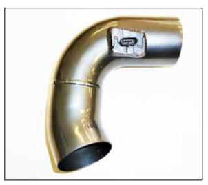
12. Remove the mass air sensor from the factory air filter housing and install it into the AEM intake tube and secure with the provided hardware.
