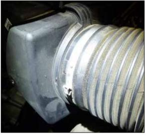
6. Cut the one-time use clamp the secures the intake hose to the intake plenum and then remove the intake tube from the vehicle.
