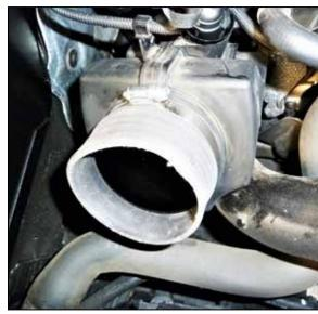
11. Install the provided coupler onto the plenum and secure with the provided hose clamp.
