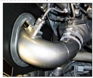
13. Install the intake tube through the hole in the heat shield and then into the coupler. Do not secure the hose clamp at this time. Connect the mass air sensor electrical connection.
