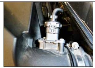
3. Release the locking tab and then disconnect the mass air sensor electrical connection.
