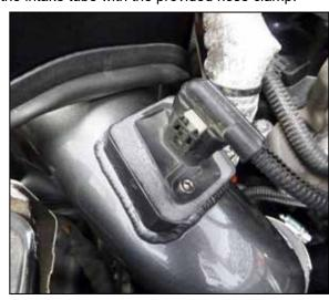
14. Connect the mass air sensor electrical connection.
