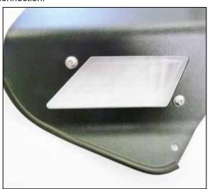
15. Install the provided edge trim onto the heat shield lid as shown using the provided super glue. Install the AEM window into the lid using the provided hardware and spacer.
