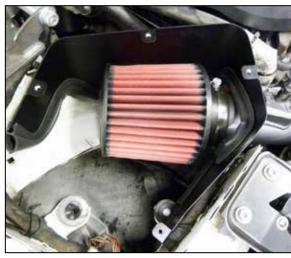
13. Install the air filter onto the intake tube and secure with the provided hose clamp. Adjust the tube and filter assembly for best fit and then secure the intake tube with the provided hose clamp.
