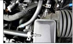
3. Release the two spring clamps that secure the vent hoses and then disconnect the vent hoses from the intake system.
