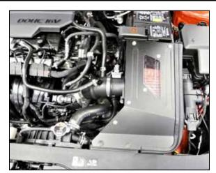
18. Install the lid onto the heat shield and secure with the provided hardware.
