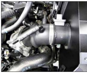
14. Install the hose/maf housing assembly onto the throttle body and into the heat shield. Adjust the maf housing so the holes line up and secure with the provided hardware. Adjust the hose for best fit and then secure with the provided hose clamps.
