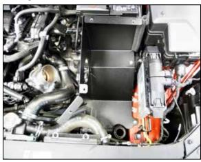
11. Install the heat shield assembly onto the rubber mounted studs and secure with the provided hardware.
