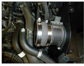
13. Install the provided straight coupler onto the mass air sensor and secure with the provided hose clamp.
