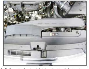
2. Pull up the fresh air intake duct to dislodge it from the mounting brackets and then remove it from the vehicle.
