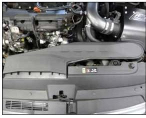
21. Reinstall the Fresh air intake duct.
