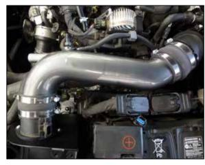
15. Install the intake tube into the hump coupler and then into the straight coupler, adjust for best fit and then secure with the provided hose clamps.
