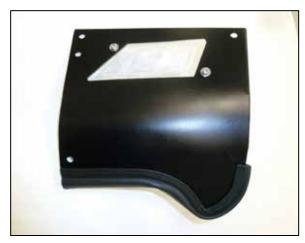
19. Install the AEM window into the heat shield lid with the spacer between the window and the lid. Secure the assembly with the provided hardware. Install the 11.5 section of edge trim onto the lid as shown.
