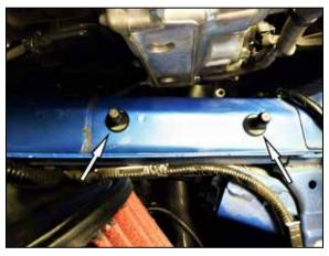
20. Install the mounting posts into the frame rail where shown.
