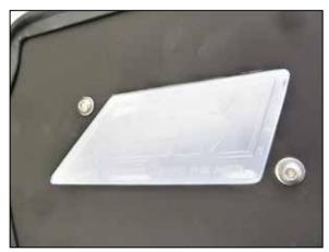
18. Install the AEM window into the heat shield using the provided hardware.
