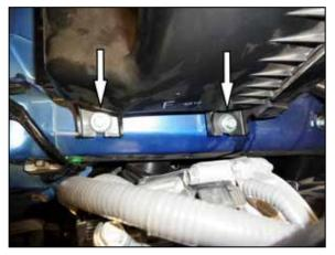
5. Remove the two bolts that secure the air filter housing to the inner fender.
