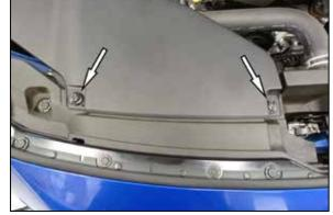
2. Release the centers of the retaining pins that secure the fresh air duct to the core support, remove the pins and then remove the fresh air duct from the vehicle and set aside to be reinstalled later.
