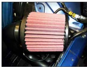
15. Install the AEM air filter onto the intake tube and secure with the provided hose clamp.
