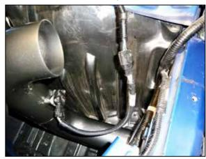
14. Connect the provided MAF extension harness to the factory maf harness and to the MAF sensor.
