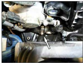
7. Loosen the hose clamp that secures the turbo inlet tube to the turbo and then remove the tube from the vehicle.
