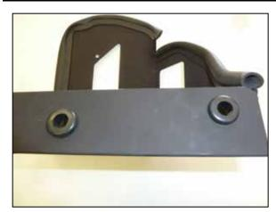
17. Install the mounting grommets into the holes in the bottom of the heat shield.
