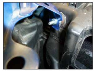
4. Remove the nut that secures the air filter housing vibration damper to the core support.
