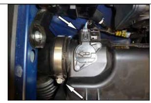
3. Loosen the hose clamp that secures the factory intake tube to the air filter housing. Disconnect the mass air sensor electrical connection.
