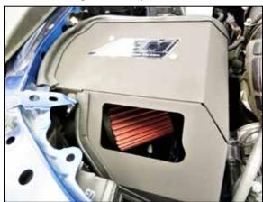
22. Install heat shield assembly onto the mounting studs and vibration mounts, secure with the factory mounting nuts.
