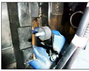
10. Remove the lower factory vibration damper and replace with the damper provided. Secure with the factory nut.
