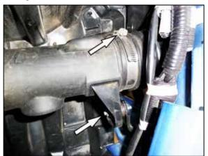
6. Remove the nut that secures the lower portion of the factory intake tube to the vibration damper and then loosen the hose clamp securing the intake tube to the turbo inlet tube. Remove the factory intake tube from the vehicle.
