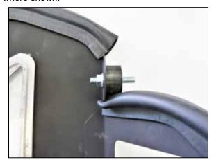
21. Install the provided vibration damper onto the heat shield using the factory nut.
