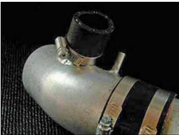
f. Trim hose to 1.5". Attach blow off valve (BOV) hose to inlet pipe and rotate as necessary for proper fit. Secure with hose clamp.
