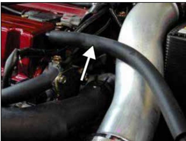
h. Locate the crankcase breather hose.
