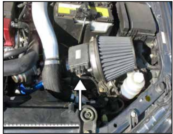
p. Reattach MAF sensor harness. Some vehicles may require that you remove approximately 2" of wire loom tape to create more slack to route the MAF harness.
