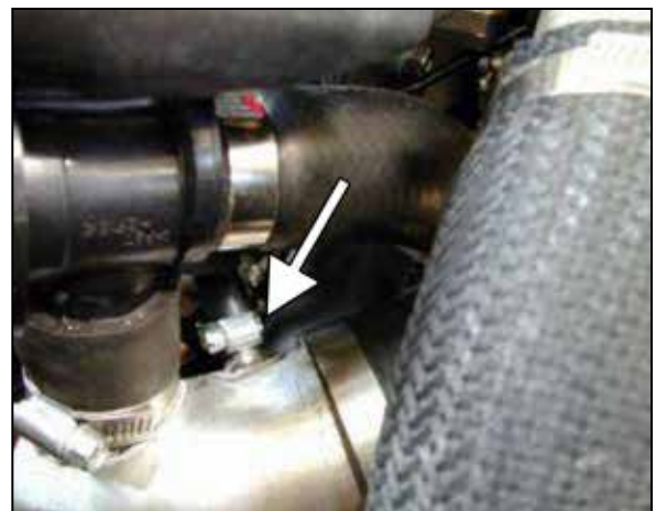
i. Secure the factory breather hose to the nipple with the provided hose clamp.
