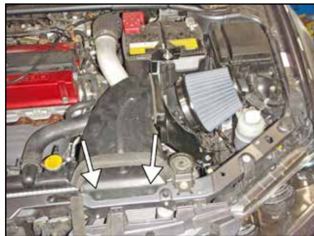
s. Re-attach the factory inlet scoop and secure with the original push-in tabs.
