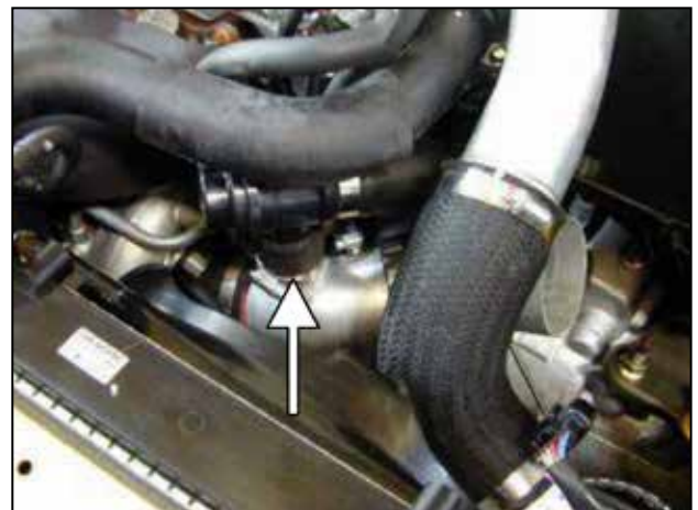
g. Insert BOV outlet into the BOV hose. Make sure you rotate the BOV toward the firewall, so that it clears the coolant hose.
