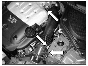
c. Loosen the hose clamps as shown. Unplug the Mass Air Flow (MAF) sensor and detach the MAF wiring harness from the sensor.
