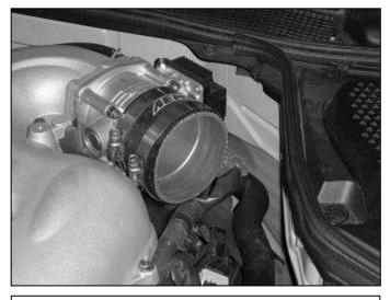
j. Install the coupler onto the throttle body. The 3" side attaches to the throttle body. Tighten the coupler to the throttle body with hose clamp no. 48.
