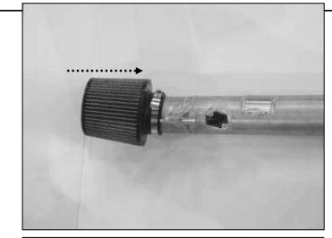
I. Attach the air filter element to the end of the inlet pipe. Secure with hose clamp.
