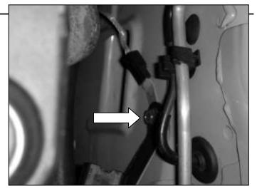
i. Install the ground strap mounting bolt. The heat shield bracket installs on top of the ground strap.
