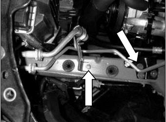
h. Remove the A/C line bracket bolts shown in the picture. The second bolt is located nearest the motor. Be careful not to damage the A/C lines.
