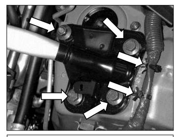
a. Remove the bolts and nut holding the strut tower bar in place. Unclip the electrical wiring loom connections.
