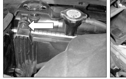
f. Secure the heat shield at the radiator with the factory screw. Be careful not to over tighten.
