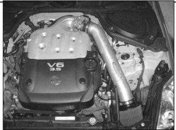
AEM<sup>®</sup> intake system installed
