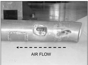
k. Install the MAF sensor into the pipe with factory hardware. Be careful not to damage the sensor during installation. Note the air flow direction.
