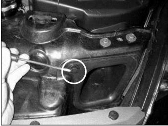
d. Pop out and remove the plastic fastener on the front air duct. Unsnap the duct and slide it forward. Remove the duct from the vehicle.
