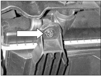
j. Loosen and remove fan shroud mounting screw. This screw will be reused in a later step.
