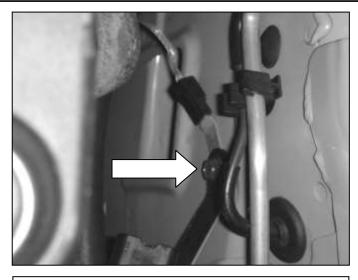
i. Loosen and remove the ground strap bolt. The strap will be reinstalled during the installation process.
