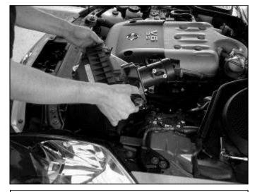
g. Gently pull directly upward on the air filter housing assembly until it unsnaps from its mounts and remove it from the engine bay.
