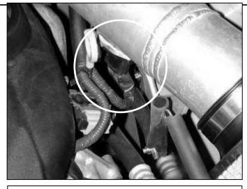
p. Check for clearance around the MAF sensor. Reattach the MAF sensor wire harness, ensure there is adequate clearance.
