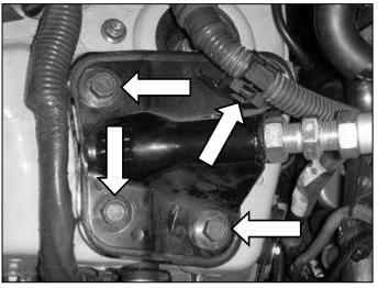
b. Remove the bolts and nut on the passenger side. Remove the remaining bolts to the strut bar. Remove the strut bar.
