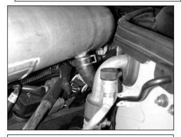
n. Reattach the crankcase breather hose to the inlet pipe. Secure with the factory spring clamp.
