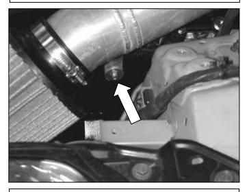
o. Align the mounting bracket to the rubber mount installed in step 3b. See diagram below for proper assembly.
