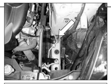
h. Install the other A/C mounting bolt. The heat shield bracket installs on top of the A/C mount.
