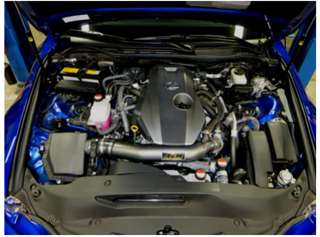
AEM INTAKE INSTALLED
