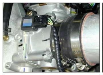
f. Install the silicone coupler over the throttle body and hose clamps but do not tighten hose clamps.
