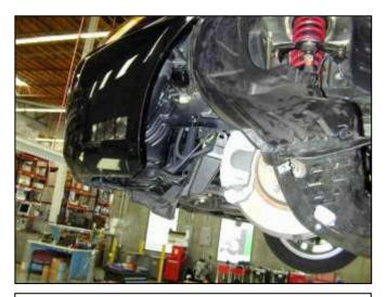
i. Raise the front of the vehicle with a jack. Refer to your owner's manual for proper jack and jack stand placement to properly support vehicle. Support your vehicle using properly rated jack stands before wheel removal or while working under the vehicle. **NEVER WORK UNDER A VEHICLE WITHOUT USING JACK STANDS.**
