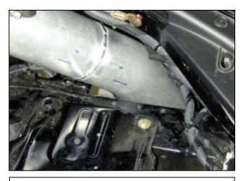
e. Install the AEM<sup>®</sup> intake pipe by routing the filter (large) end of the pipe through the opening in the engine bay between the battery location and the fender. Be sure to have the mounting bracket on the intake facing the front of the car and use rags to prevent the pipe from being scratched.
