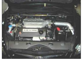
AEM® intake system installed
