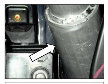
j. Reinstall the plastic battery under-tray, the battery, and the battery tie down bracket. Do not install the plastic battery cover. Check for proper clearance between the battery and the intake pipe. Use the supplied zip-ties to make sure no wires are in contact with the intake system.
