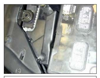
c. Remove the plastic shielding in front of the battery by pulling the two plastic snaps out and lifting straight up on the shield.
