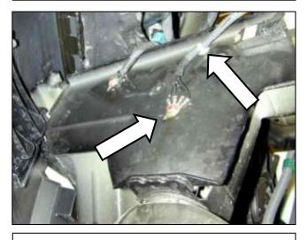
m. Remove the bolt securing the rearward grounding block and unhook the wire clips securing the wires to the chassis.
