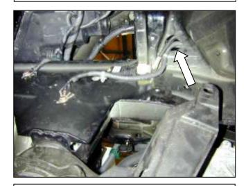
n. Route the wire through the hole located a few inches rearward in the chassis. Then reconnect the grounding block where it was originally located and secure the wires using the supplied zip-tie. The hole locating stud will bend back.
