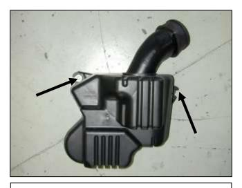
k. On automatic transmission equipped cars the stock intake resonator looks like the one pictured above. Remove the two bolts holding it in place. **NOTE: The second bolt is located on the top front side of the resonator.**
