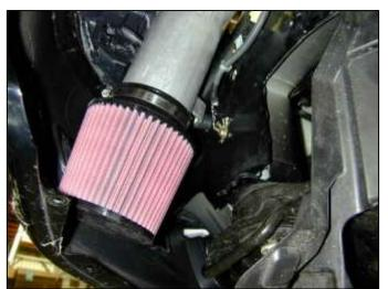
h. Install the AEM<sup>®</sup> air filter on to the end of the inlet tube. Push the air filter over the inlet pipe until the stop in the filter is reached. Install one hose clamp to secure the filter onto the inlet pipe. Once fitment is checked, tighten the hose clamp.
