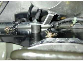
g. Guide the bracket on the intake pipe over the stud on the rubber mount. Once aligned, install the supplied washer and nut onto the stud. Do not tighten until fitment is complete.
