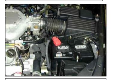
Factory air box system installed
