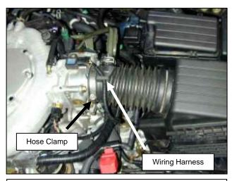
e. Loosen the hose clamp on the throttle body and unhook the wiring harness.
