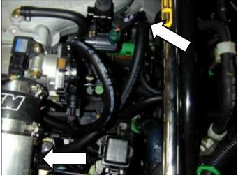
i. Install the supplied ½" breather hose between the intake pipe and the valve cover as shown.
