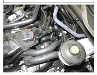
i. Once the charge pipe is in its proper location, insert the upper end into the throttle body coupler. Do not tighten the hose clamp yet. You may reattach the heater hoses into their clips at this time.
