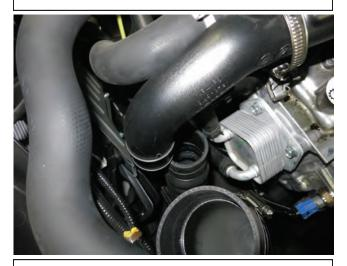
m. Loosen the hose clamp securing the charge pipe to the intercooler hose. Then, pull the charge pipe from the hose.
