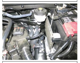
o. Reinstall the battery heatshield.
