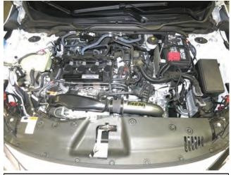
STOCK CHARGE PIPE INSTALLED
