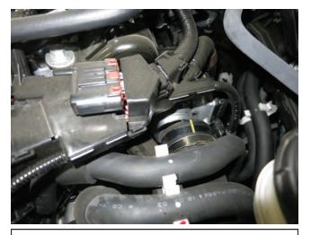
k. Loosen the hose clamp securing the charge pipe to the throttle body. Then, pull the hose end off of the throttle body.
