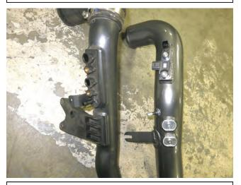
c. Using the stock hardware and an 8mm socket, transfer the MAP and IAT sensors from the stock charge pipe to the AEM charge pipe.
