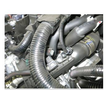
c. Disconnect the manifold absolute pressure (MAP) sensor and intake air temperature (IAT) sensor harnesses.
