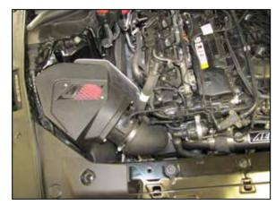
18. Reinstall the intake system into the vehicle and secure to the intake plenum, reconnect the inlet air temperature sensor electrical connection.
