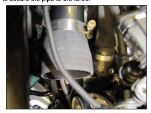
13. Using the provided T-bolt, install the provided step coupler onto the lower charge pipe. NOTE: It will be necessary to loosen the nut on the clamp completely to allow the clamp to slide onto the coupler, it is a tight fit to secure the coupler tightly against the tube bead. It is easier to install the coupler and clamp onto the tube on the bench before the tube is installed into the vehicle.
