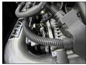
15. Reconnect the two sensor electrical connections. Note: Due to manufacturer tolerance, the wiring harness may need to be adjusted to allow for enough slack in th wiring harness.
