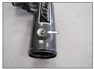
10. Install the 1/8npt pipe plug into the water injection port. **NOTE:** be sure to use pipe tape or other pipe sealant on the threads of the plug (not supplied).
