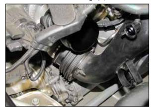
8. Release the locking clip that secures the charge pipe to the turbo outlet, separate the charge pipe from the turbo and remove it from the vehicle.
