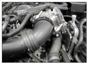
6. Remove the two bolts that secure the factory charge pipe to the throttle body.
