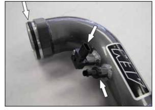
9. Remove the two sensors and O-ring from the factory charge pipe and install them onto the AEM charge pipe as shown.
