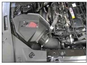
3. Disconnect the inlet air temperature sensor electrical connection and then remove the complete air intake system from the vehicle. **NOTE: AEM-21-875DS intake system pictured.**
