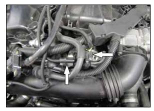
4. Disconnect the electrical connections from the two sensors installed into the factory charge pipe.
