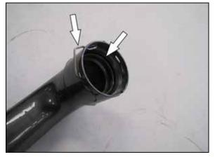
11. Remove the retaining clip and O-ring from the lower section of the factory charge pipe and install them onto the AEM charge pipe as shown.
