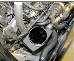
17. Reinstall the turbo inlet plenum being sure the retaining clip snaps into the groove to secure the plenum to the turbo. Reconnect the CCV vent to the plenum.
