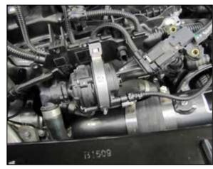
16. Reinstall the coolant pump clamp.
