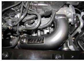
14. Install the upper charge pipe into the coupler and then into the throttle body, secure the tube to the throttle body with the provided hardware and then secure the coupler with the T-bolt clamp.
