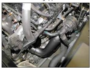
12. Install the AEM lower charge pipe onto the turbo outlet, be sure that the locking clip engages to secure the pipe to the turbo.
