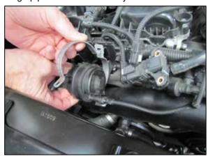
7. Remove the bracket that secures the coolant pump. This pump will not be removed, removing the bracket will aid in the charge pipe removal.
