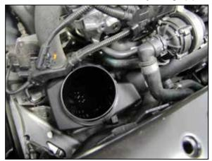
5. Disconnect the CCV vent from the turbo intake plenum, release the retaining clip that secures the plenum onto the turbo inlet and then remove the plenum from the vehicle.
