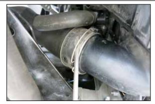
3. Using a screwdriver, remove the retaining clip that secures the lower charge pipe quick connect coupler.
