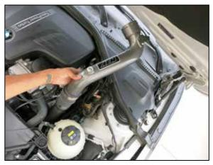
14. Feed the charge tube into the vehicle and align with the throttle body and intercooler connections.
