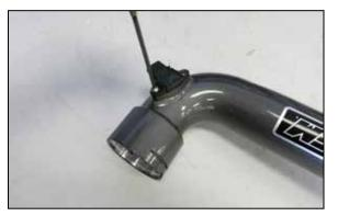
9. Install the pressure sensor into the AEM charge tube and secure with the provided hardware.
