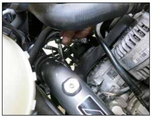
17. Connect the lower charge tube quick connect coupler to the inter cooler, Adjust the tube and coupler for best fit and then secure the T-bolt clamps on the coupler.
