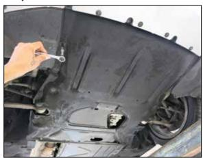
19. Reinstall the lower valence onto the vehicle and secure with the factory hardware.
