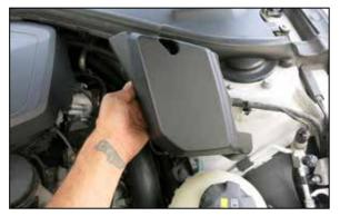
4. Remove the screw that secures the ECU cover and then remove the cover from the vehicle.
