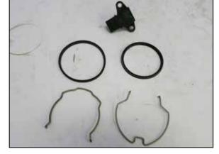
8. Remove the pressure sensor, retaining clips and O-rings from the factory charge tube.
