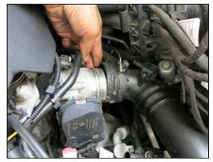
6. Disconnect the CCV hose from the factory charge tube clip. Release the retaining clip that secures the upper quick connect coupler to the throttle body and then separate the charge tube from the throttle body.
