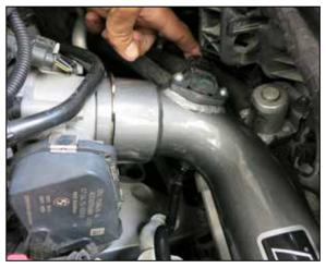
15. Snap the throttle body side quick connect coupler onto the throttle body. Be sure the retaining ring is fully locked. Reconnect the pressure sensor electrical connection.
