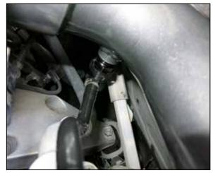
16. Connect the CCV pipe to the fitting installed into the AEM charge tube.
