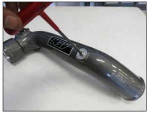
11. Install the provided 1/8npt pipe plug into the accessory port. Be sure to use pipe sealant or Teflon tape on the threads.
