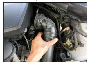
7. As the factory charge tube is removed from the vehicle, disconnect the CCV pipe from the underside of the charge tube and then completely remove the charge tube from the vehicle.
