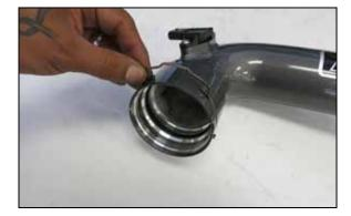
10. Install the O-rings and retaining clips into the AEM charge pipes.
