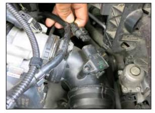
5. Disconnect the pressure sensor electrical connection.
