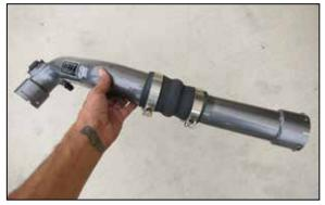
13. Assemble the two sections of charge tube with the provided hump coupler and clamps loosely to allow for adjustment.
