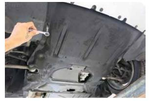
2. With the vehicle secured on jack stand or lift, remove the screws that secure the lower valence to the vehicle and then remove the valence.
