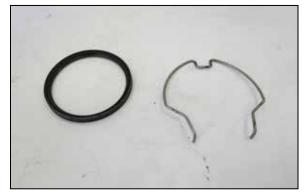
12. Remove the O-ring and locking clip from the factory charge pipe.
