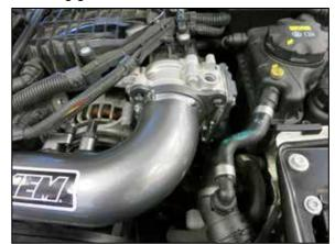
8. Using a flat blade screwdriver, unlock the clip that locks the charge pipe to the turbo outlet. Remove the charge tube assembly from the vehicle.
