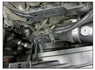
21. Reconnect the vacuum switch to the CCV line.
