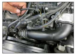
6. Disconnect the charge tube pressure and temperature sensor electrical connections.
