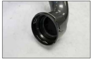
14. Install the locking clip onto the AEM charge tube as shown.
