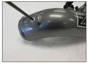
16. Install the 1/8npt pipe plug into the AEM charge pipe as shown. **NOTE: Be sure to use pipe sealant on the threads.**
