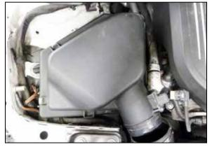
22. If not installing a AEM intake system, Reinstall the factory intake tube and air filter housing assembly.
