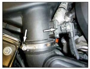
23. Reconnect the mass air sensor electrical connection and connect the intake tube to the air filter housing and secure with the factory hose clamp.
