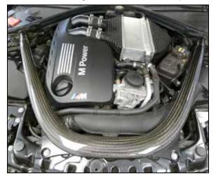
17. Reinstall the strut tower brace and covers, secure with the factory hardware.
