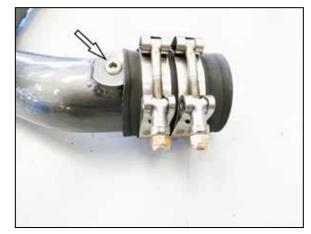
10. Install the provided 1/8npt accessory port plugs into the AEM charge tubes. NOTE: be sure to apply pipe sealant on the threads of the plugs. Install the provided couplers and clamps onto the charge tubes. NOTE: Slide the couplers all the way onto the pipes as shown as this will aid the installation of the pipes.
