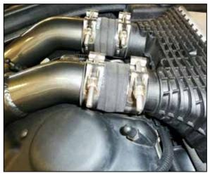
6. Remove the bolt that secures the turbo inlet pipe and then disconnect the pipe from the turbo and remove it from the vehicle.
