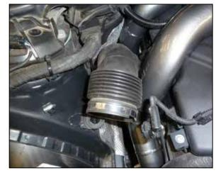
14. Install the factory intake tube onto the turbo inlet and secure with the factory clamp.
