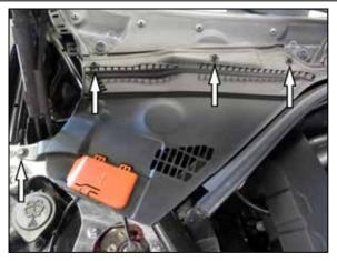
2. Remove the retaining pin and turn the three fasteners 1/4 turn counterclockwise to unlock, then remove the cover panels from the vehicle.
