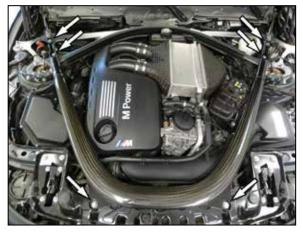
3. Remove the six bolts that secure the strut tower brace and then remove the brace from the vehicle.
