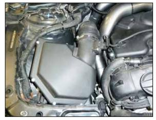
15. Reinstall the air filter housing, secure the intake tube with the factory hose clamp and reconnect the maf sensor electrical connection.
