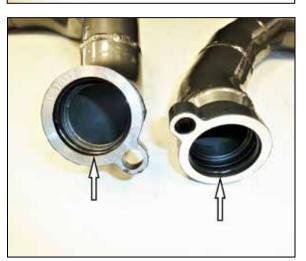
9. Remove the O-rings from the factory charge tubes and install them into the AEM charge tubes.
