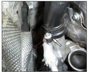
8. Remove the bolts that secure the factory charge tubes to the turbo and then remove the charge tubes from the vehicle. NOTE: The following size wrenches can be used to remove the TORX bolts, T50 TORX, 5/16" 12-point wrench, 8mm 12-point wrench.
