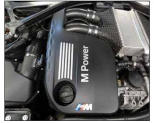
4. Remove the oil fill cap and then lift off the engine cover. Reinstall the oil fill cap or use a towel to keep debris from entering the engine.
