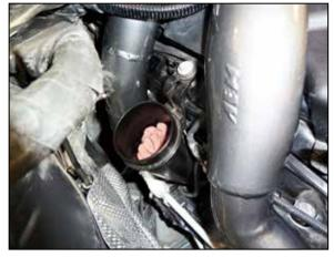
13. Reinstall the turbo inlet and secure with the factory hardware.
