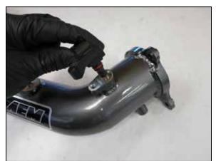
12. Install the pressure sensor into the AEM charge tube and secure with the provided hardware.
