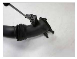
9. Remove the screw that secures the pressure sensor into the factory charge pipe and then remove the sensor from the pipe.
