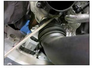
5. Using a flat blade screwdriver, release the retaining clip from lower factory charge pipes lower connection.
