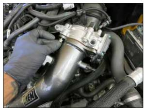
16. Secure the pipe to the throttle body with the hardware provided.
