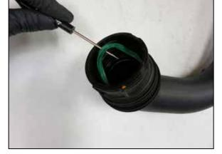
8. Remove the factory O-ring from the factory charge pipe.
