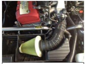
b. Re-install the intake tube/air filter assembly.
