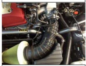
d. Re-connect AIT sensor wire, clip sensor wires back to intake the intake tube.
