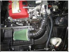
a. Unclip and remove the airbox cover.
