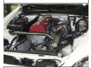
f. AEM strut bar installed with an AEM intake (not included).
