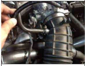
c. Re-connect the vent tube and secure with the clamp.
