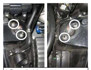
d. Remove the 4 damper nuts.
