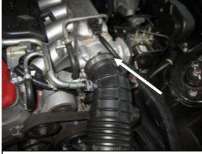
b. Loosen the clamp holding the intake tube to the throttle body.
