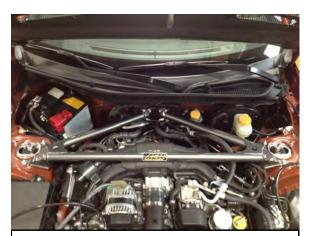
c. Install the AEM Strut Tower Bar, and replace all factory hardware.
