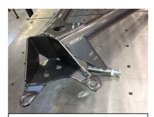
b. Assemble the included nut and bolt on the brake master cylinder brace.
