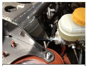
d. **By hand**, unscrew the brake master cylinder bolt until it **just touches** the brake master cylinder. Using a 17mm wrench, tighten the nut against the strut bar.
