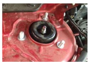
a. Place the (6) washers over the 6 strut studs.
