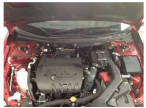
a. With the car on the ground, use a 14mm socket to remove the (6) strut top nuts.
