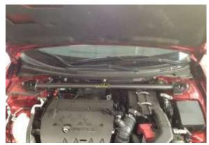
b. Install the AEM Strut Bar, and using a 14mm socket, replace the strut tower nuts.
